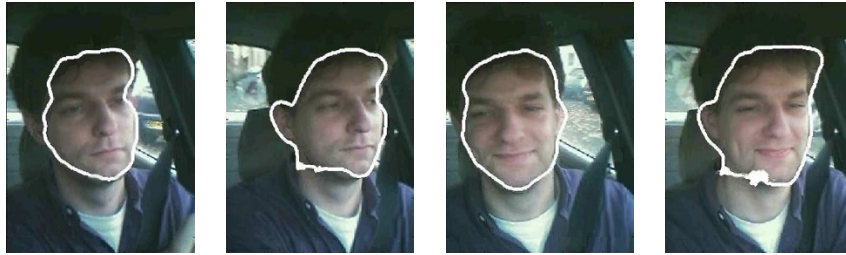
FIGURE 10: Contour tracking applied to driver’s face extraction, using the weighted gradient (skin chroma being the feature of interest). Randomly chosen images from a video sequence.
