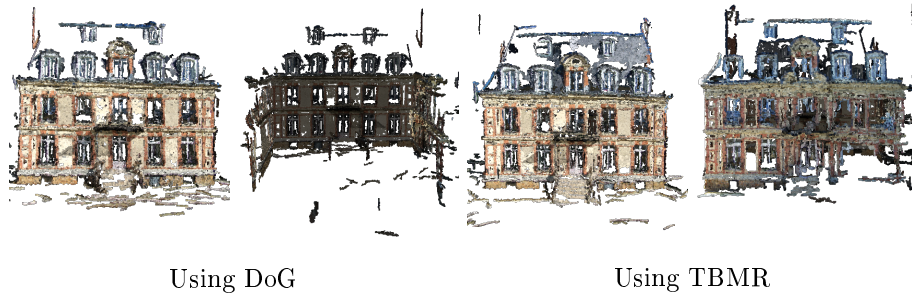
Figure 2.22: Three dimensional reconstruction from multiple view stereo images, using DoG or TBMR as interest points. Notice that the back facade of the castle is lost using DoG because of lack of correct correspondences, while TBMR recovers a more complete 3D.
