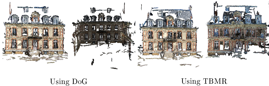
Figure 2.22: Three dimensional reconstruction from multiple view stereo images, using DoG or TBMR as interest points. Notice that the back facade of the castle is lost using DoG because of lack of correct correspondences, while TBMR recovers a more complete 3D.
