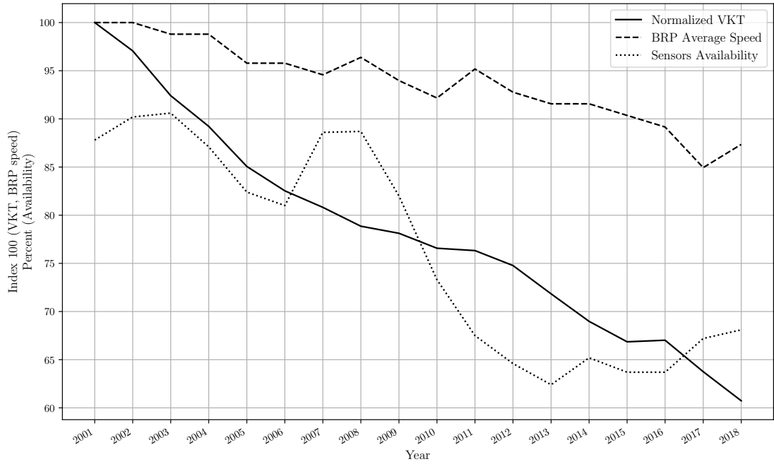
Figure 2.8 – Normalized VKT and BRP Speed over TPIM arterial network. Monthly averages, business days, 07:00-21:00. Indexed on January 2001 values. Sensors availability, in %.
