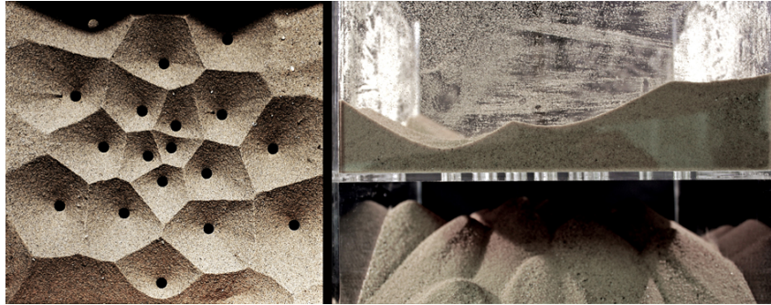
Figure 2.4 – Sand creates naturally constant slope surface, the sand is added at specific points and the crest lines create a Voronoi diagram [114] (picture: sandworks ).
