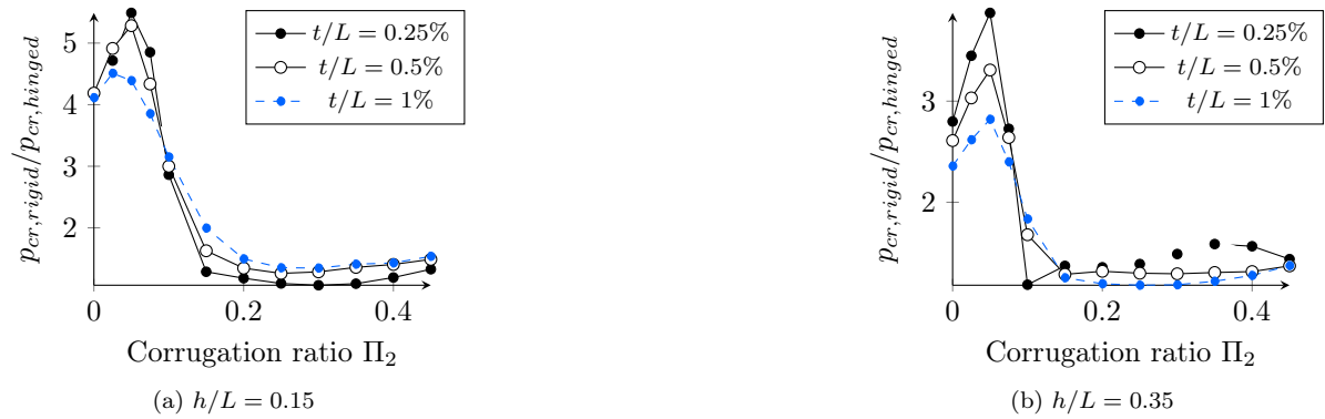
Figure 7.40 – Ratio of the linearised buckling loads for the rigid and hinged plates configurations
