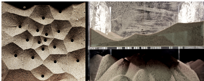
Figure 2.4 – Sand creates naturally constant slope surface, the sand is added at specific points and the crest lines create a Voronoi diagram [114] ( picture:sandworks ).
