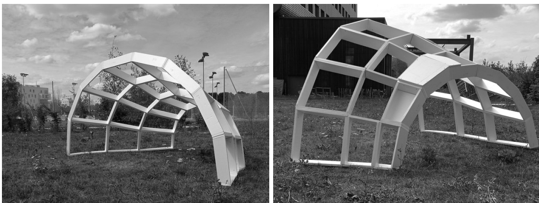
Figure 4.43 – A model of a canal surface with planar quadrangles used for bracing.
