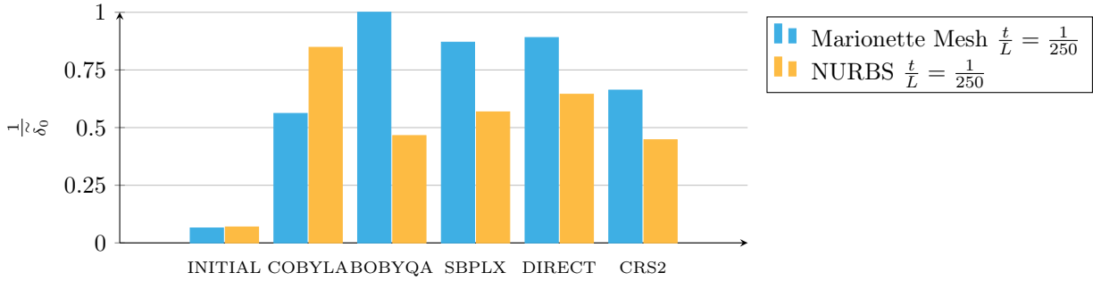
Figure 6.25 – Optimal values found for the minimisation of displacement under self-weight ( \frac{t}{L} = \frac{1}{250} ).
