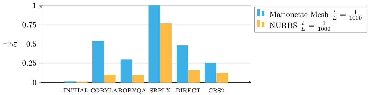
Figure 6.23 – Optimal values found for the minimisation of displacement under non-symmetrical load ( \frac{t}{L} = \frac{1}{1000} ).
