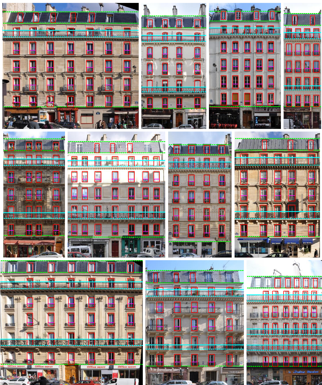
Figure 3.13: Example results of the proposed algorithm. Green lines separate sky from roof, roof from facade and facade from shop. Balconies are outlined in magenta or cyan. Note the variety of alignment patterns supported by the algorithm (top right). Typical errors are presented in the bottom row. In these images window columns can be missed due to the randomized, non-exhaustive search of the structure space. In the second and third images, our grammar does not model complex-enough patterns of the facade, like vertical misalignment of windows and middle-size balconies.
