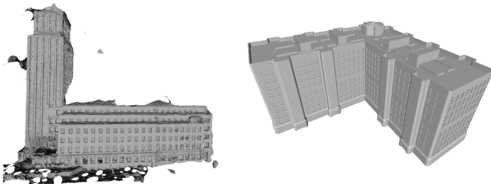
Figure 1.2: An output of a 3D reconstruction pipeline (left) and a geometric building model (right). The model contains a low number of polygons and is free from noise. Additionally, it features perfect alignment of architectural elements. We are interested in models that contain semantic information (not presented in the image) in addition to geometry.
