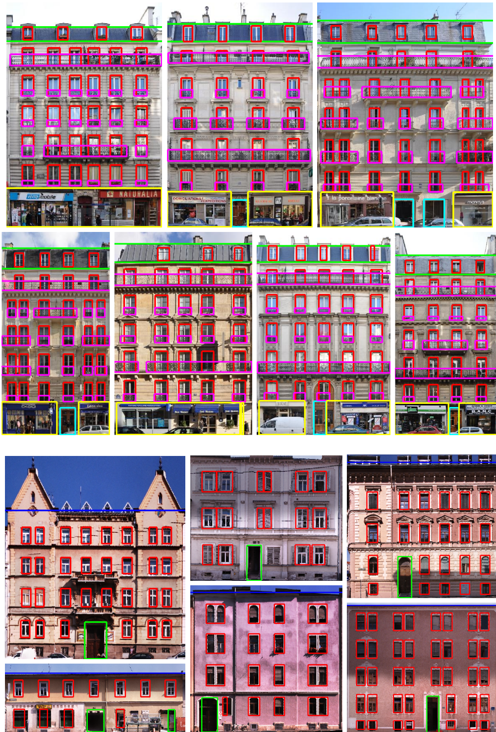
Figure 4.6: Example parsing results on the ECP dataset (top and middle) and on the Graz50 dataset (bottom). Green lines separate sky from roof and roof from facade. Balconies are outlined in magenta, shops in yellow, and doors in cyan. Note the variety of alignment patterns supported by the algorithm (top right). Typical errors are missed doors and missed roof windows.
