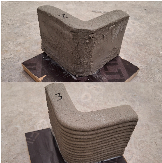
Fig. 20. Smooth sample (top) and heterogeneous sample (bottom) used for evaporation measurements.
