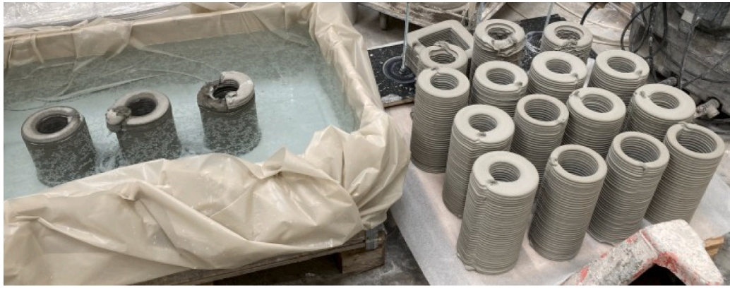
Fig. 2. Printed specimens for compressive strength measurements.
