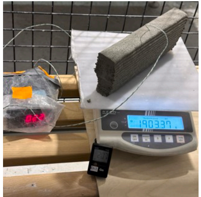
Fig. 10. Experimental setup to measure the evaporation rate and monitor the surface and air temperature.
