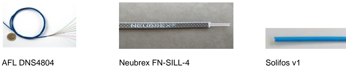
Figure 3. Pictures of the various Optical Fibers Cables tested on VeRCoRs mockup
