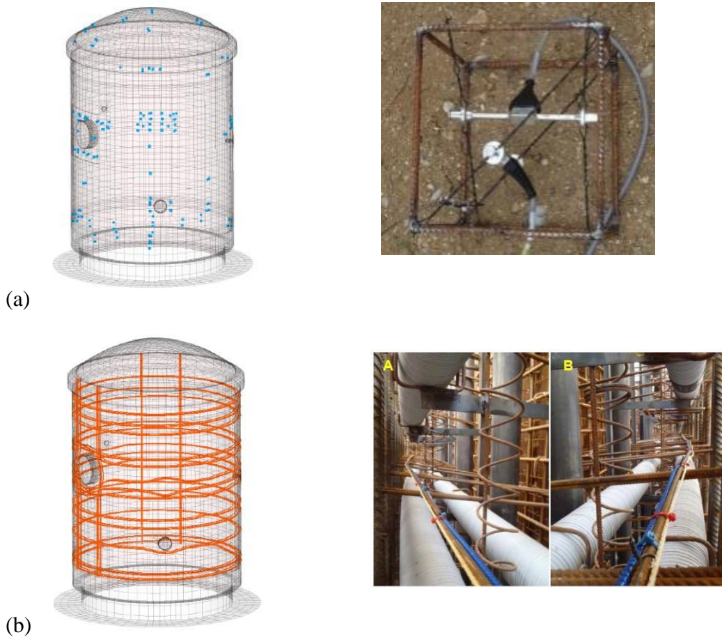
Figure 2. Local and distributed concrete strain measurement systems on VerCoRs Mockup – VWSG at the left (blue color on the drawing) and Optical Fiber cables on the right (orange color on the drawing)
