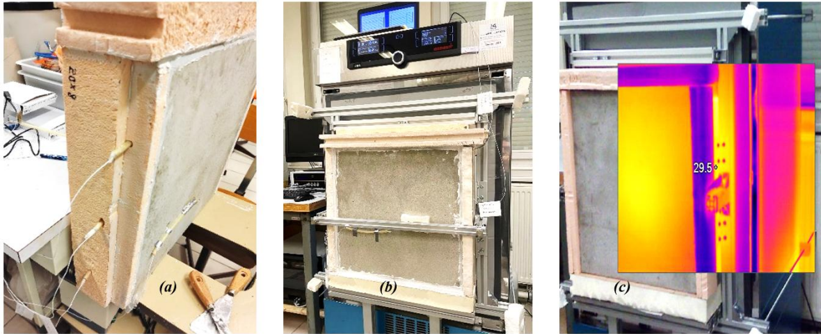
1 2 Figure 2. (a) Wall preparation with sensors; (b) Experimental setup; (c) IR image of the wall 3 to check uniform heat transfer and prevent heat losses.
