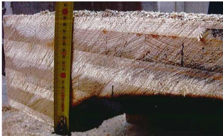
Figure 2.1 Residual cross section of the Test-1 floor
