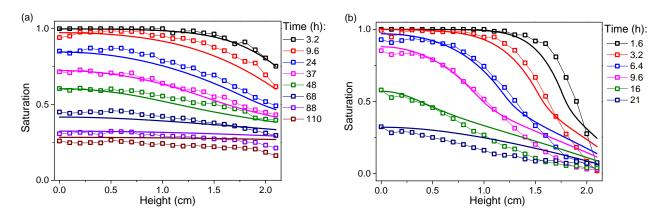
Figure 6: Bound water distribution over time as measured (symbols) at different times (see legend) during drying under (a) air flux at 50% RH and (b) dry air flux (data extracted from Figure 5), and predictions (continuous lines) from of the diffusion model with a two-step diffusion coefficient (see text).
