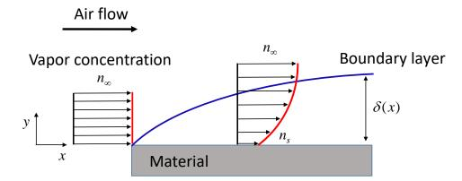
Figure 2: Boundary layer of vapor concentration resulting from air flow along a material surface.  $\delta$  is the characteristic distance of diffusion of vapor through air from the interface, i.e., roughly the distance over which one observes the main variations of the RH from the surface of the material
