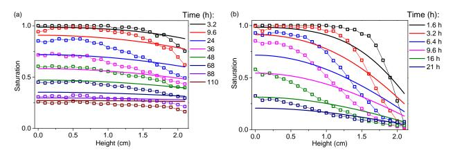
Figure 7: Bound water distribution over time as measured (symbols) at different times (see legend) during drying under (a) air flux at 50% RH and (b) dry air flux (data extracted from Figure 5, and predictions (continuous lines) from of a simple diffusion model with a constant diffusion coefficient  $6 \times 10^{-9}$  m<sup>2</sup> s<sup>-1</sup>.
