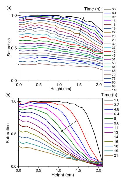
Figure 5: Bound water distribution over time during drying under different conditions: (a) Air flux at 50% RH ( $\delta = 29 \text{ mm}$ ), (b) Dry air flux ( $\delta = 6.6 \text{ mm}$ ). The air flux is applied along the top surface situated on the right in the graph. The successive profiles are obtained from MRI measurements at different times during drying. For each profile the measurement duration is 1.6 h.
