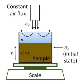
Figure 3: Scheme of the principle of a controlled sorption kinetics test.
