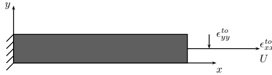
FIGURE 10.2: Uniaxial tensile test on a bar of length L .
