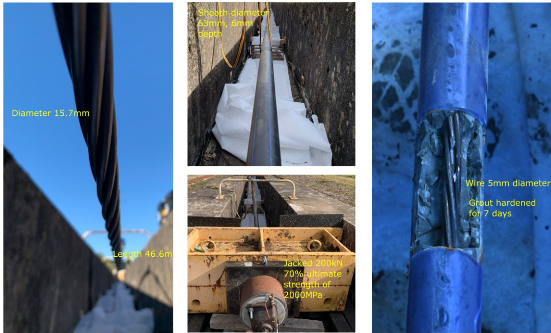
FIGURE 3 Set up of the experimental bench
