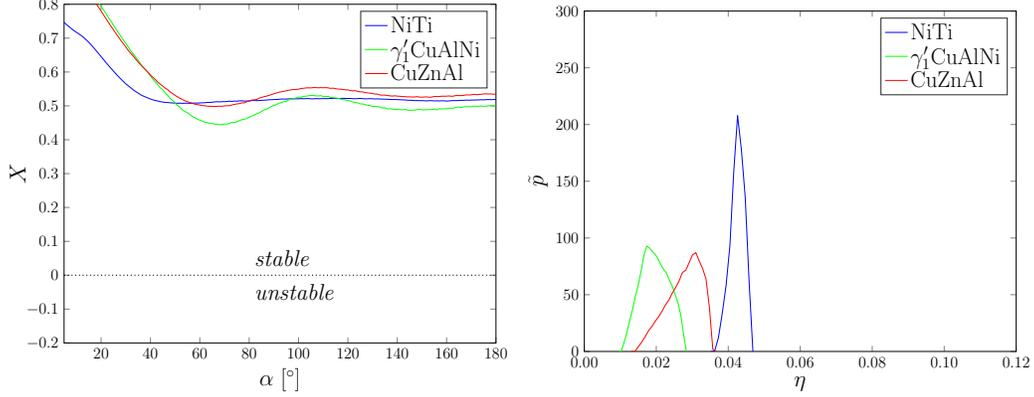
Figure 10: (left) Localization criterion vs wobble for a fiber texture  $\langle 111 \rangle \parallel \mathbf{u}_1$  in several materials. (right) Densities of the transformation strain  $\eta$  for a fiber texture  $\langle 111 \rangle \parallel \mathbf{u}_1$  (with  $10^\circ$  wobble) in several materials.
