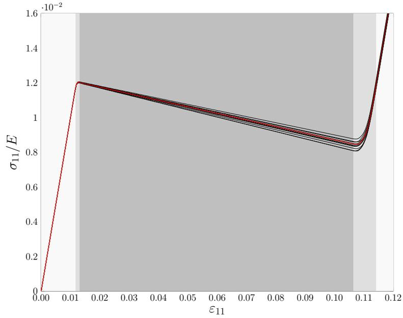
Figure 11: stress-strain curves for  $\langle 111 \rangle \parallel \mathbf{u}_1$  textures with  $10^\circ$  wobble: numerical solutions for examples of textures with 100 grains (black), analytical solution (red).
