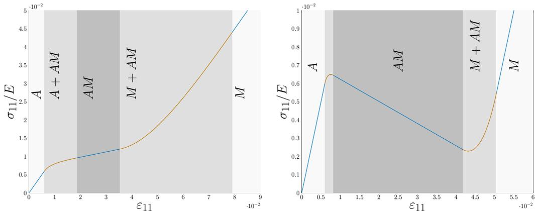
Figure 2: Stress-strain curve for a model texture with a density  $\tilde{p} = 1/(\eta^+ - \eta^-)$ ;  $\eta^+ = 0.05$ ,  $t = 0$ ,  $\gamma = 0.0003$ ,  $g_0 = 0.001$ ,  $b = 0.4$ . Cases  $\eta^- = 0.02$  (left) and  $\eta^- = 0.04$  (right).
