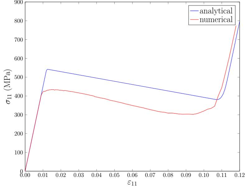
Figure 13: stress-strain curves for  $\langle 111 \rangle \parallel \mathbf{u}_1$  textures with  $10^\circ$  wobble: numerical solutions for a texture with 100 grains (red), analytical approximation (blue).
