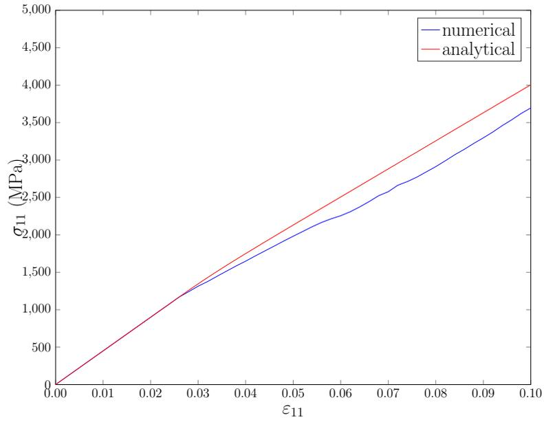
Figure 15: stress-strain curves for a  $\langle 111 \rangle \parallel \mathbf{u}_1$  texture with  $10^\circ$  wobble in CuAlNi: numerical solutions for 100 grains (red), analytical approximation (blue).
