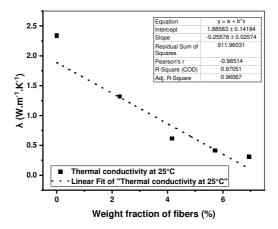
FIGURE 5: Evolutions of the thermal conductivity of mortars at 25 °C as a function of the weight fraction content of miscanthus fibers
