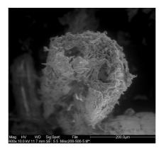
FIGURE 1: SEM pictures of the micronized miscanthus fibers used in this study
