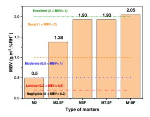
FIGURE 6: Moisture Buffer Value of various mortars including miscanthus fibers and comparison with the Nordtest classification.
