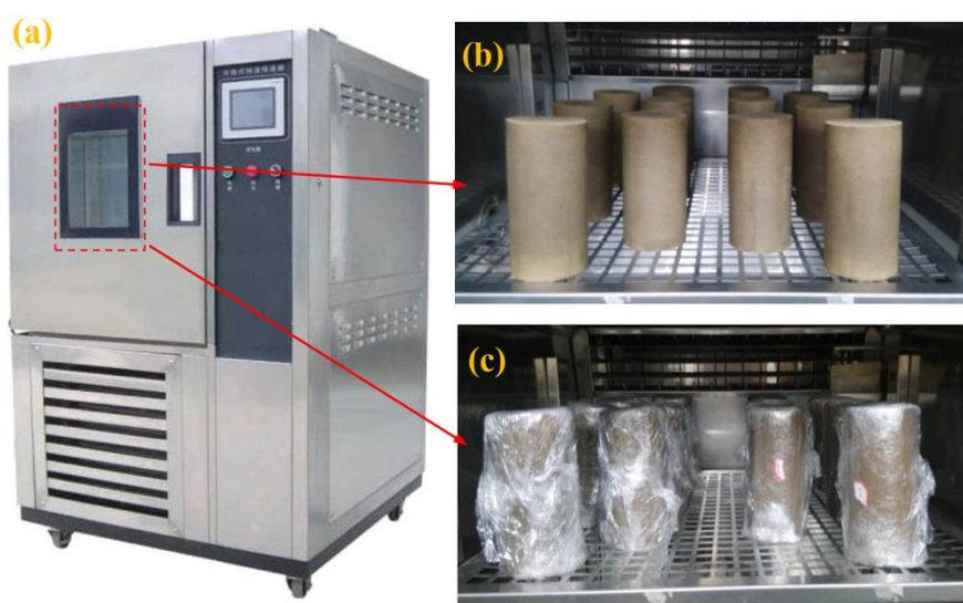
172 173 Fig. 4 WDFT process in the temperature and humidity control box: (a) test apparatus, (b) drying 174 process, and (c) freezing-thawing (FT) process
