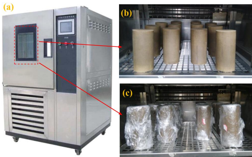
Fig. 4 WDFT process in the temperature and humidity control box: (a) test apparatus, (b) drying process, and (c) freezing-thawing (FT) process
