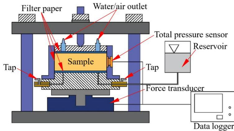
Fig. 2. Layout of the constant-volume cell for swelling pressure tests
