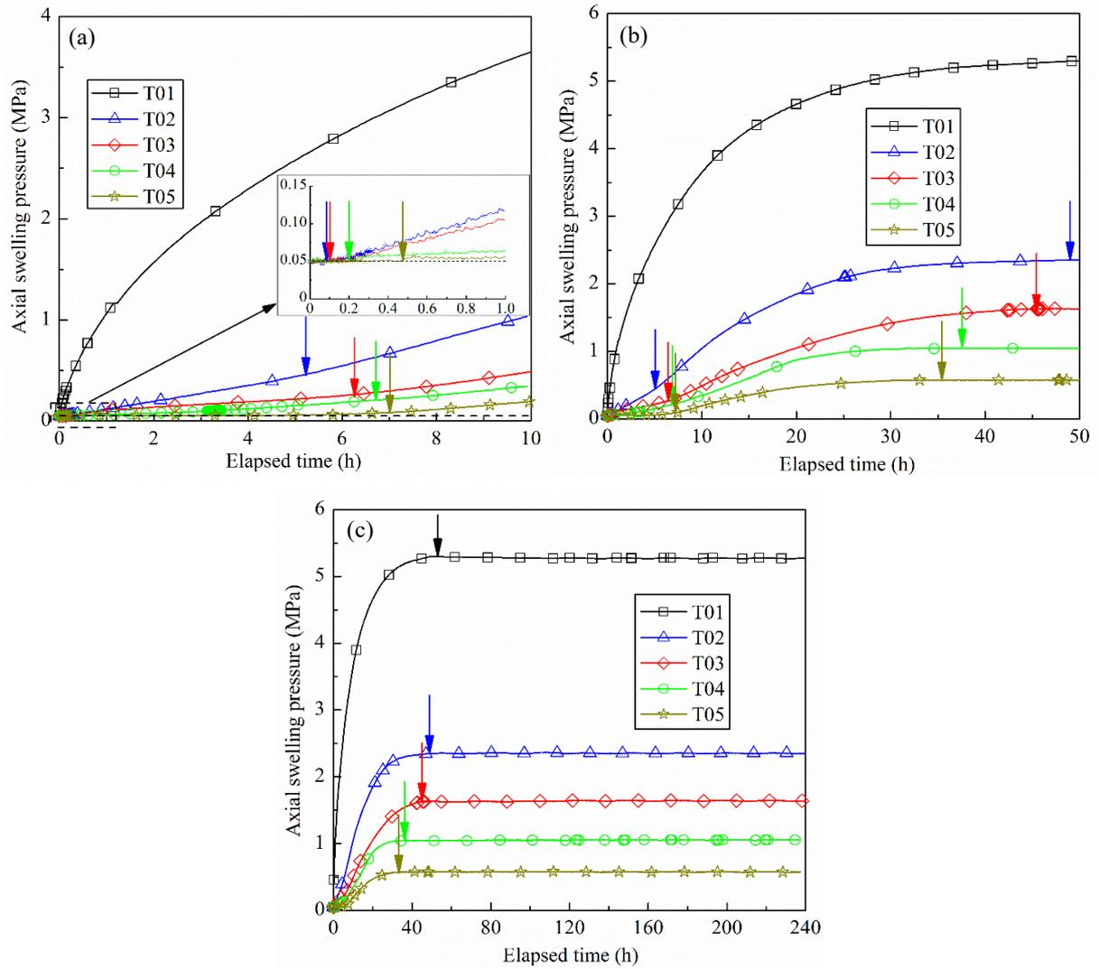
**Fig. 4.** Evolution of axial swelling pressure (a) in the first 10 h, (b) in the first 50 h, and (c) for the whole test duration. Note: the curves in the figure are drawn according to all the measurement points but only a few symbols in each curve are plotted for distinction purpose
