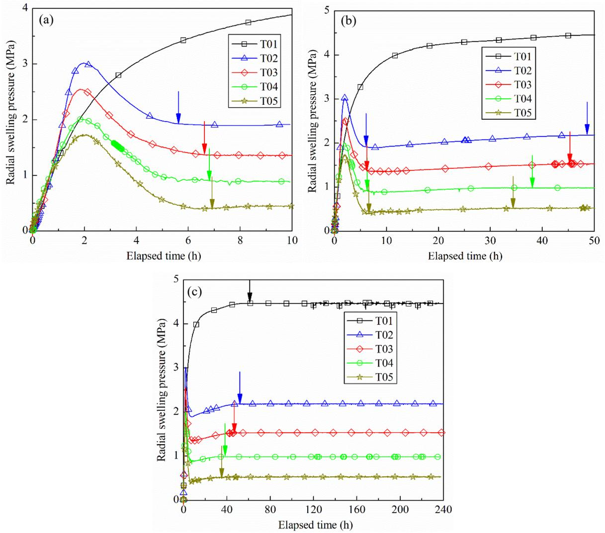
**Fig. 5.** Evolution of radial swelling pressure (a) in the first 10 h, (b) in the first 50 h, and (c) for the whole test duration
