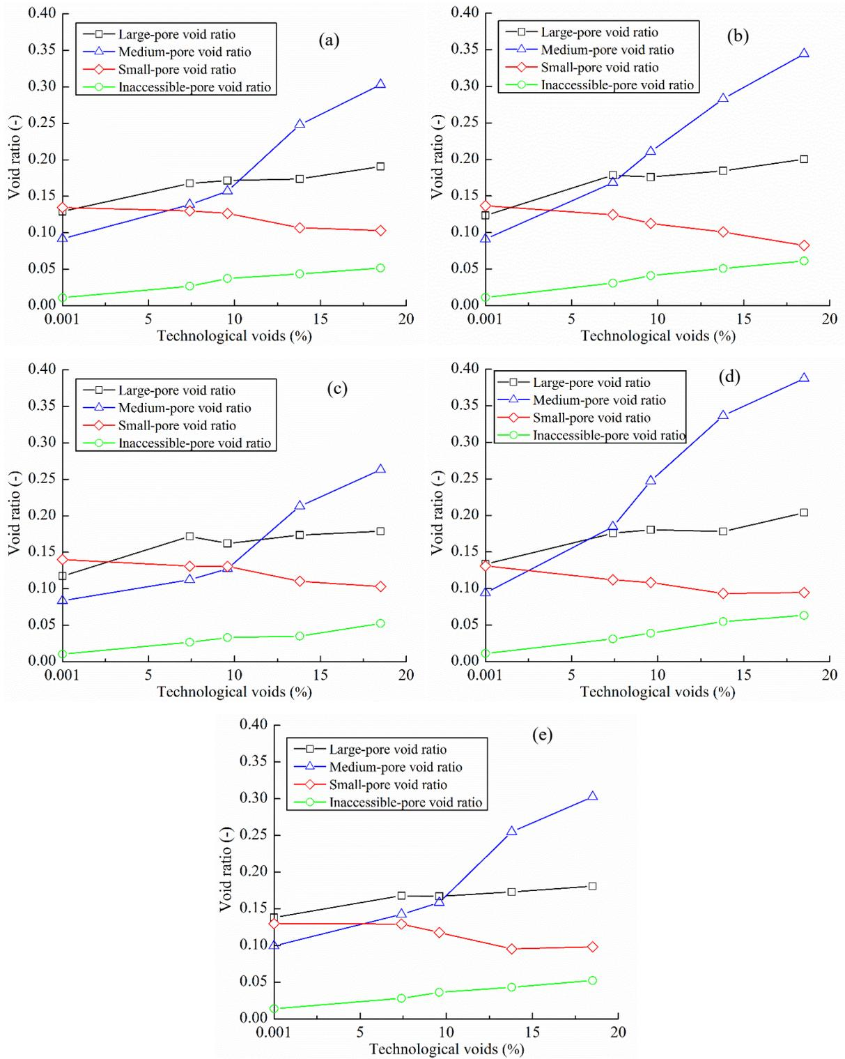
**Fig. 11.** Changes in inaccessible-pore, small-pore, medium-pore and large-pore void ratios with technological voids for (a) layer I, (b) layer II, (c) layer III, (d) layer IV and (e) layer V
