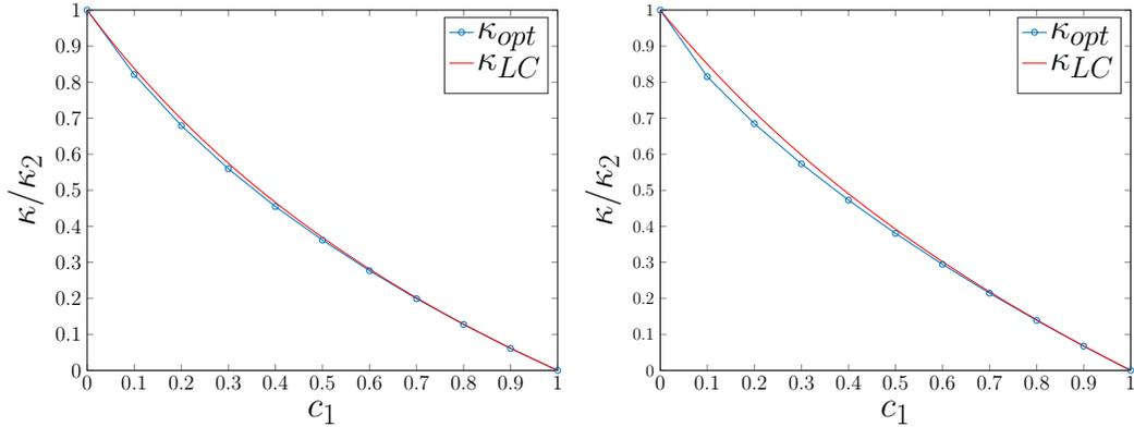
Figure 11: Effective resistivity as a function of the volume fraction  $c_1$ , for  $m = 2$  (left) and  $m = 5$  (right). Square tessellation.
