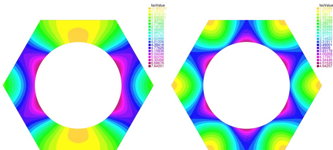
Figure 14: Maps of the energy density  $w_2/\sigma_2\|\bar{e}\|^{m+1}$  (left) and symmetrized energy density  $w_{2,sym}/\sigma_2\|\bar{e}\|^{m+1}$  (right) for a circular inclusion in a periodic hexagonal cell with  $m = 2$ ,  $c_1 = 0.4$ ,  $\theta = 0$ .
