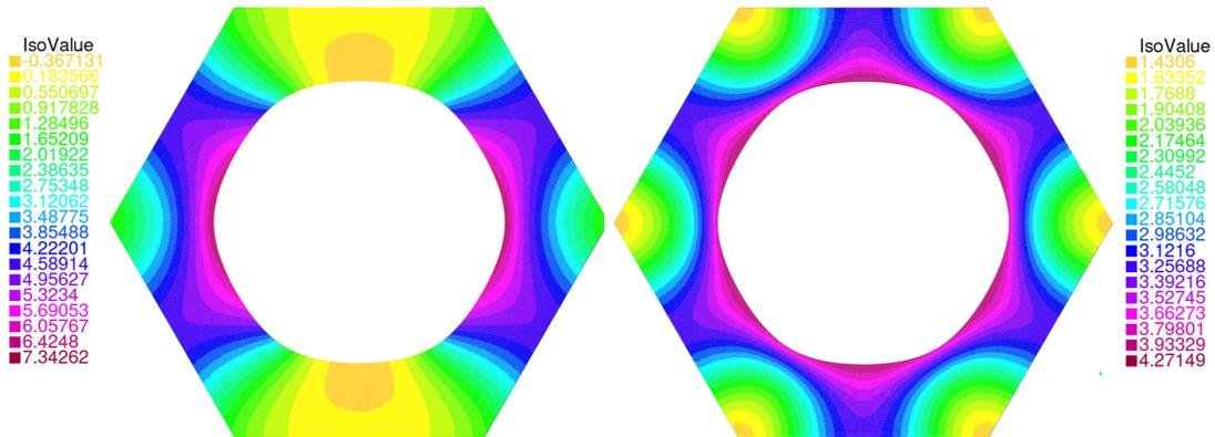
Figure 15: Maps of the energy density  $w_2/\sigma_2\|\bar{e}\|^{m+1}$  (left) and symmetrized energy density  $w_{2,sym}/\sigma_2\|\bar{e}\|^{m+1}$  (right) for the optimized inclusion in a periodic hexagonal cell with  $m = 2$ ,  $c_1 = 0.4$ ,  $\theta = 0$ .
