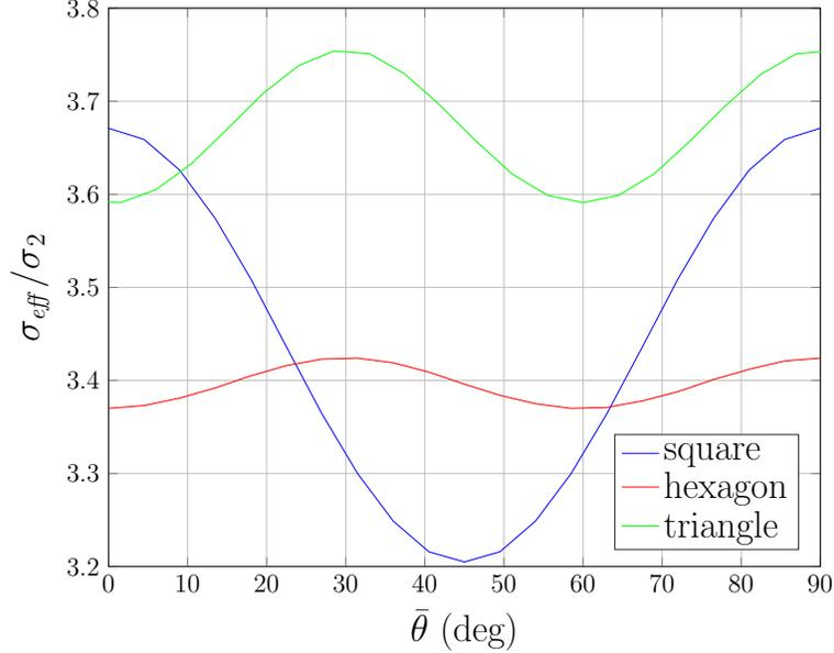
Figure 6: Effective resistivity in the loading direction  $\theta$  for circular perfectly conducting inclusions in a power-law matrix with nonlinearity index  $m = 2$ . The volume fraction  $c_1$  of the inclusions is set to 0.3. Three tessellations are considered: square, hexagonal, triangular.
