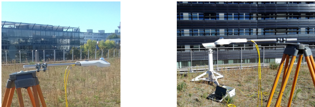
Figure 21. CNR4 Net Radiometer
