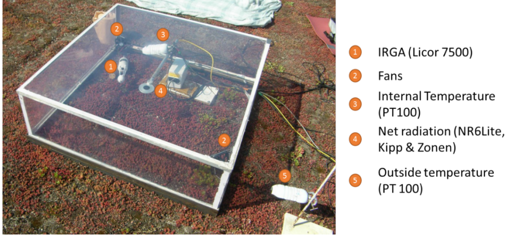
Figure 7. Evapotranspiration chamber, (Ramier et al., 2015)
