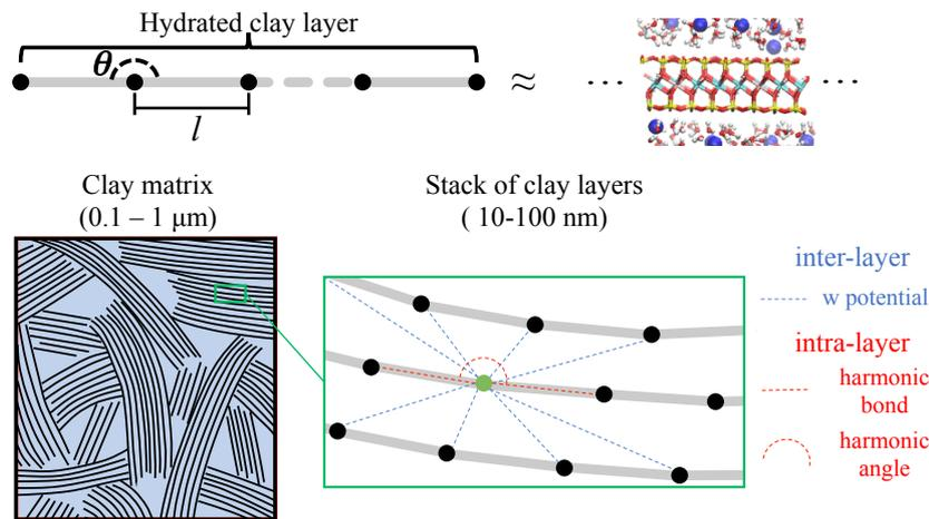
Figure 1: Schematic representation of the 2D granular mesoscale model of clay. Chains of particles represents flexible hydrated clay layers. Intra-layer energy is modeled by nearest neighbors interactions with harmonic bonds and angles. Inter-layer energy is modeled by the double well pair potential ( $w$  potential, see Fig. 2 and Tab. 1) capturing the 1W and 2W hydration states.
