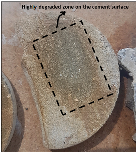
Fig. 4. Cement specimen after carbonation for 30 days at 20 MPa and 90°C.
