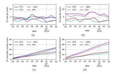
**Figure 7.** Evapotranspirations (ETs) and water level variations (dH) in the internal water storage for lysimeters 1, 3, and 4 (a) and lysimeters 6, 3, and 4 (b) during a summer period (24 June to 3 July 2018). (c,d) show cumulative values for ETs and |dH|, respectively, for lysimeters 1, 3, 4, and lysimeters 6, 3, and 4.
