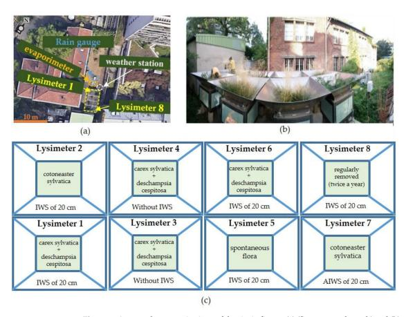
**Figure 2.** A top and panoramic views of the site in figures (**a**) (Source: google earth) and (**b**), respectively. The figure (**c**) illustrates the positions and the scientific names of vegetation in each lysimeter.
