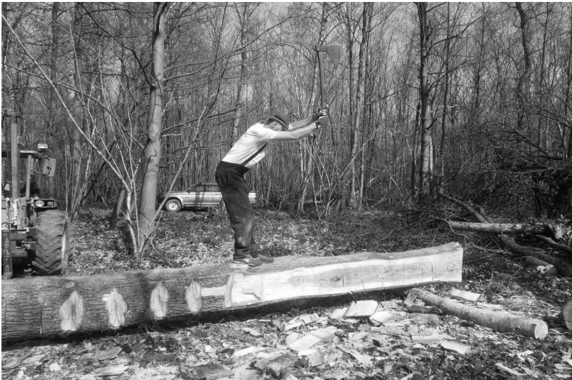
Fig. 2 Squaring an oak log by severing fibre and splitting (Photo Florian Carpentier) Severing the fibre is done first every 50 cm by two axe cutting Splitting a long 50 cm chips parallel to wood grain in then achieved
