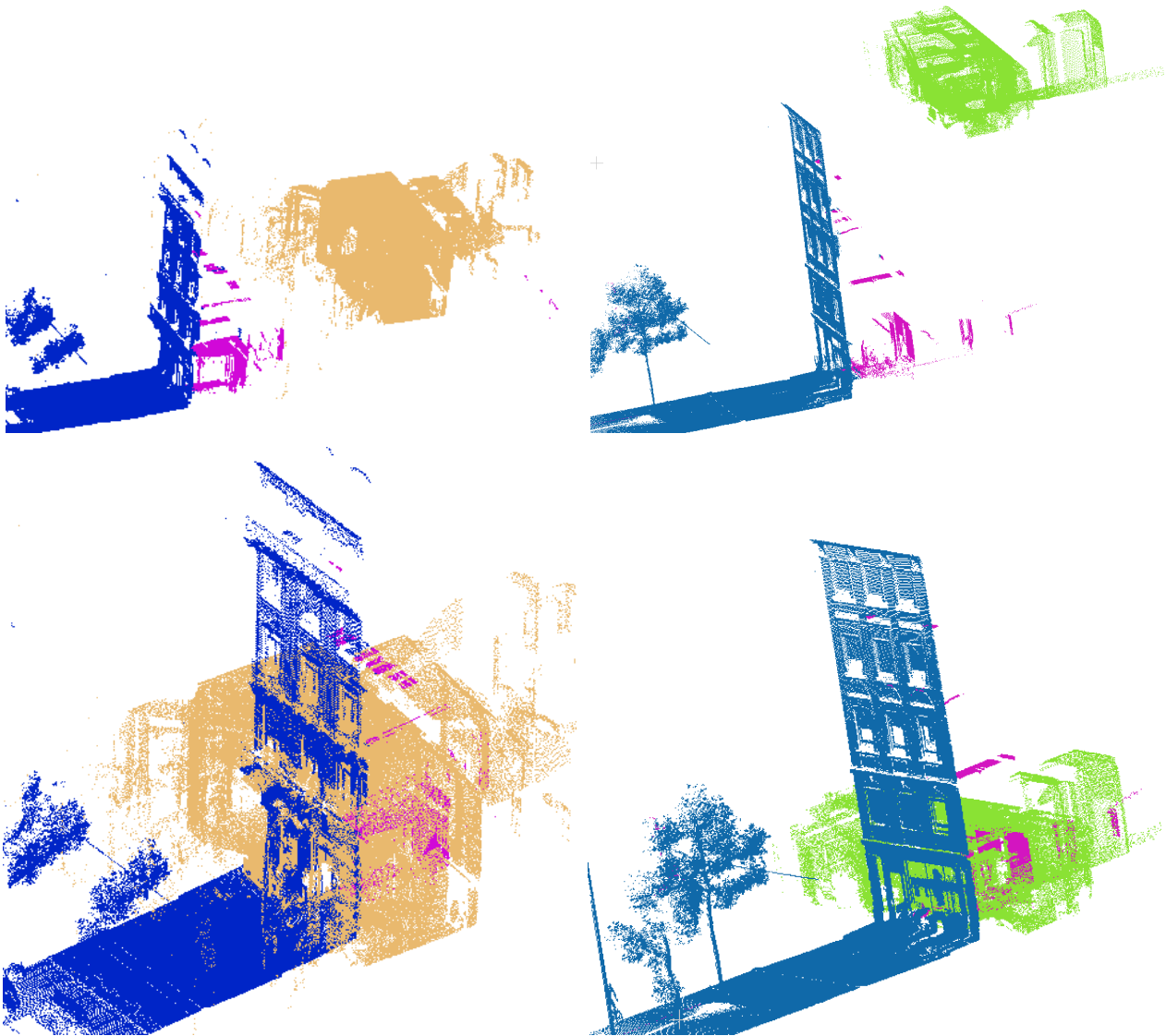
Figure 12. Result of the test of our algorithm on two pairs of indoor/outdoor scans, Top: the initial position of each pair, Bottom: The position of each pair after registration, pink points represent the indoor points detected from the outdoor scans.
