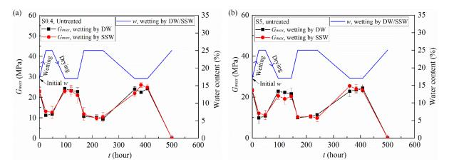
Fig. 8. G<sub>max</sub> changes during wetting-drying cycles for untreated soil: (a) S0.4; (b) S5.
