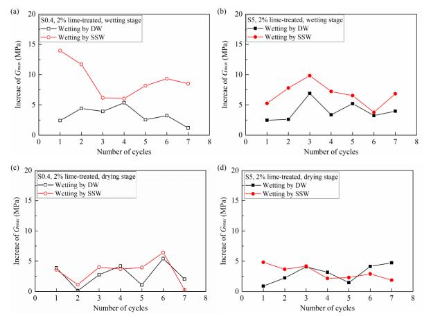
Fig. 10. Increase of  $G_{max}$  with wetting-drying cycles.
