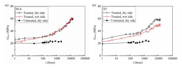
Fig. 6. Evolutions of small strain shear modulus after compaction: (a) S0.4; (b) S5.
