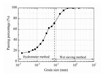
Fig. 1. Grain size distribution of the tested soil.
