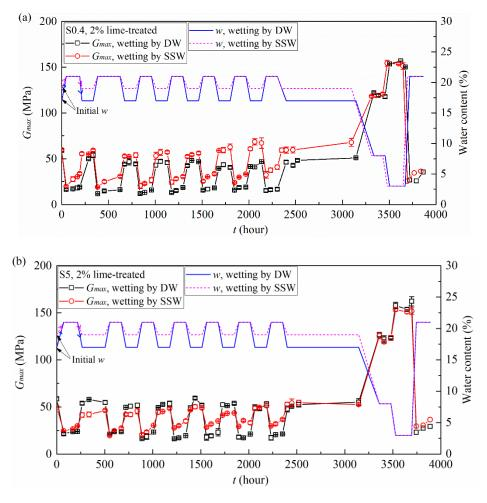
Fig. 9. G<sub>max</sub> changes during wetting-drying cycles for lime-treated soil: (a) S0.4; (b) S5.
