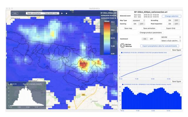
Demonstrator of the ENPC X-band Radar Platform, with the zoomed view over the Bièvre Valley on May 22, 2018, 11AM-1PM UTC. The hot spot corresponds to 26 mm of 2h cumulative rainfall over the BIEV subcatchment, situated just in between the three rain gauges (JOUY3, SYGAM and VER1 sub-catchments), the maximum per pixel is above 44 mm. This is a very heterogeneous event, only 6 mm were obtained over the full rainy area of the X-band radar observations (up to 100 km radius around the ENPC).
