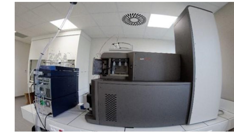
C18 chromatography and ESI+ with m/z [100-1000]
