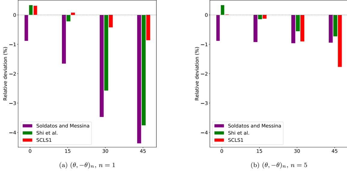
Figure 5: Relative error with respect to the three-dimensional model of the frequency parameter  $\bar{\omega} = \omega a^2 \sqrt{\rho/E_1 h^2}$  for a  $(\theta, -\theta)_n$  laminated square plate;  $a/h = 20$ ,  $E_1/E_2 = 40$ ,  $G_{12} = G_{13} = G_{23} = 0.5E_2$ ,  $\nu_{12} = 0.25$ .
