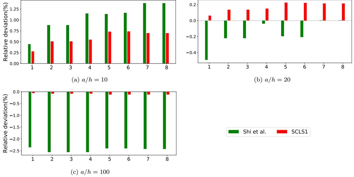
Figure 3: Relative error compared to the three-dimensional model of the frequency parameter  $\omega^* = \omega a^2 \sqrt{\rho / (E_T h^2)}$  for a clamped asymmetric plate  $(0, 90)$ . The material properties used for the calculation are  $E_L / E_T = 25$ ,  $G_{12} = G_{13} = 0.5 E_T$ ,  $G_{23} = 0.2 E_T$ ,  $\nu_{12} = 0.25$ .  $E_L / E_T = 25$ ,  $G_{12} = G_{13} = 0.5 E_T$ ,  $G_{23} = 0.2 E_T$ ,  $\nu_{12} = 0.25$ .
