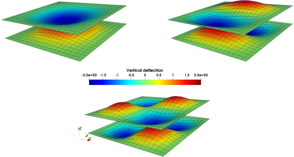
Figure 8: Representation of the 4, 5, 8<sup>th</sup> mode
