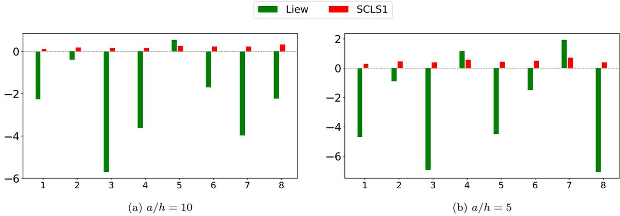
Figure 4: Relative error with respect to the three-dimensional model of the frequency parameter  $\bar{\omega} = (\omega b^2 / \pi^2) \sqrt{(\rho h / D_0)}$  ( $D_0 = \frac{E_T h^3}{12(1 - \nu_{21} \nu_{12})}$ ) for a symmetric  $(0, 90)_s$  laminate.
