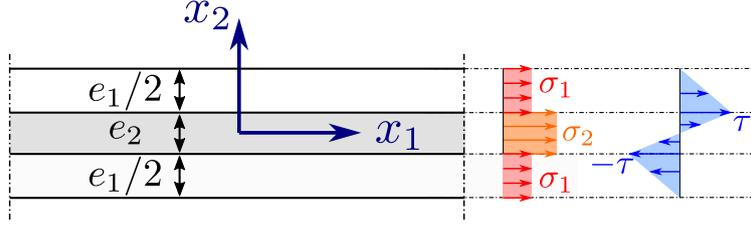
Figure 1: Geometry of the bi-material and shear-lag assumptions
