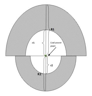
Figure 7. Geometric model of the straw collection area. The simplest circular geometry obtains when  $R_1 = R_2$  and  $r_1 = r_2 = 0$ . The two concentric non-overlapping semi annulus case has  $r_2 = 0$  and  $r_1 = R_2$
