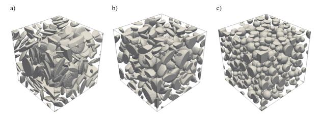
Figure 2: Examples of RSA microstructures with porosity c = 25%. Unit cells containing polydisperse (multiple size) voids with aspect ratio (a)  $\omega = 0.2$  and  $N_{pores} = 204$ , (b)  $\omega = 0.4$  and  $N_{pores} = 204$ , (c)  $\omega = 1$  and  $N_{pores} = 408$ .
