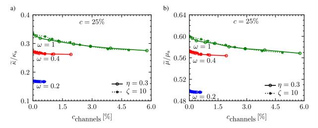
Figure 8: Effective moduli of the CRSA microstructures for fixed porosity c = 25% and various values of the pore aspect ratio  $\omega$ , coordination number  $\zeta$  and reduced channel size  $\eta$ . Solid lines:  $\eta = 0.3$ ,  $\zeta$  varies as in Fig. 6; dotted lines:  $\zeta = 10$  and  $\eta$  varies as in Fig. 7. (a) Effective bulk modulus. (b) Effective shear modulus.
