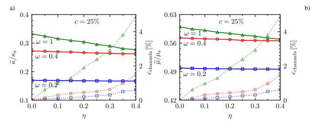
Figure 7: Effective moduli of the CRSA microstructures for fixed porosity c = 25% and coordination number  $\zeta = 10$  and various values of the pore aspect ratio  $\omega$  and reduced channel size  $\eta$ . (a) Effective bulk modulus. (b) Effective shear modulus. In both cases, the secondary right axis shows the volume fraction  $c_{\text{channels}}$  of the cylindrical channels (dotted lines) as a function of the reduced channel size  $\eta$  for the same values of c and  $\zeta$ .
