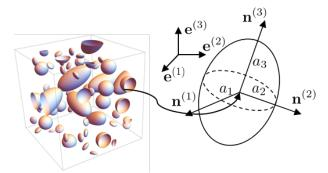
Figure 1: Example of a generated RSA microstructure, showing some of the parameters introduced in Section 3.1.
