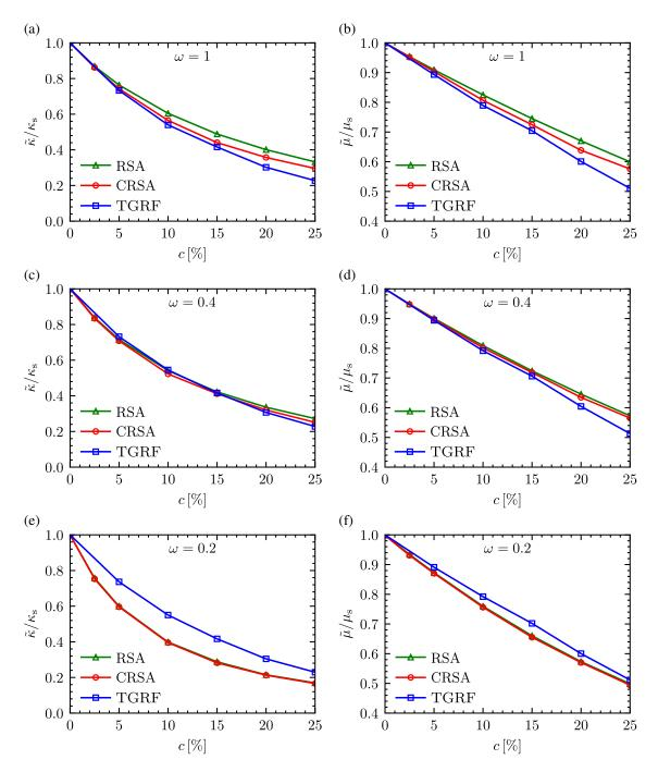
Figure 11: Effective normalized bulk  $\tilde{\kappa}/\kappa_s$  and shear  $\tilde{\mu}/\mu_s$  moduli of the RSA, TGRF and CRSA microstructures as a function of the porosity *c*, for a pore aspect ratio (a,b)  $\omega = 1$ , (c,d)  $\omega = 0.4$  and (e,f)  $\omega = 0.2$ . For the CRSA microstructures,  $\eta = 0.25$  and  $\zeta = 4$ .
