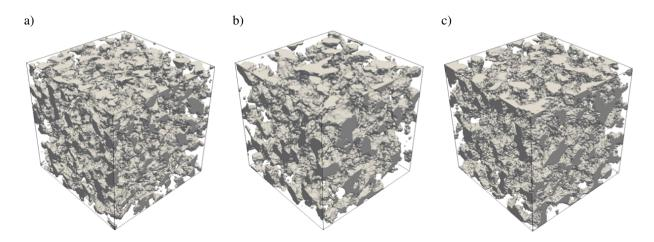
Figure 5: Examples of TGRF microstructures with porosity c = 25% reconstructed by using the two-point correlation functions of the RSA microstructures shown in Fig. 2 with void aspect ratio (a)  $\omega = 0.2$ , (b)  $\omega = 0.4$  and (c)  $\omega = 1$ .
