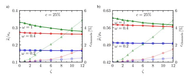
Figure 6: Effective moduli of the CRSA microstructures for fixed porosity c = 25% and reduced channel size  $\eta = 0.3$  and various values of the pore aspect ratio  $\omega$  and coordination number  $\zeta$ . (a) effective bulk modulus. (b) Effective shear modulus. In both cases, the secondary right axis shows the volume fraction  $c_{\text{channels}}$  of the cylindrical channels (dotted lines) as a function of the coordination number  $\zeta$  for the same values of c and  $\eta$ .
