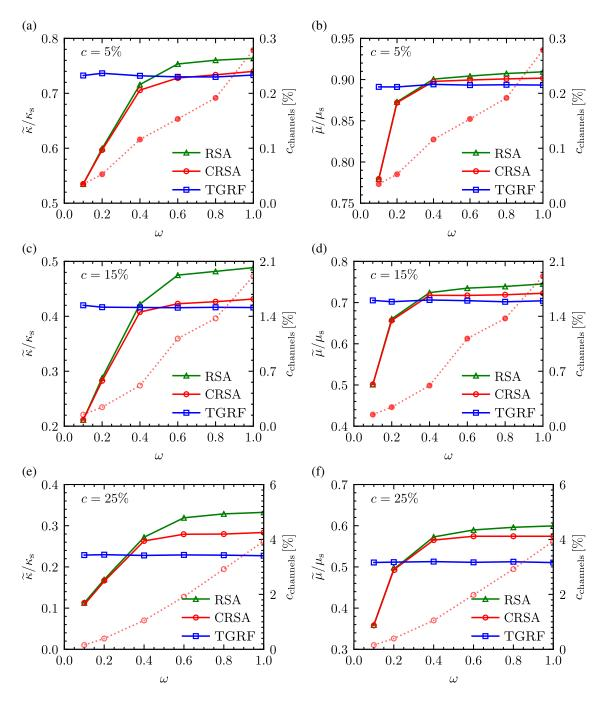
Figure 12: Effective normalized bulk  $\tilde{\kappa}/\kappa_s$  and shear  $\tilde{\mu}/\mu_s$  moduli of the RSA, TGRF and CRSA microstructures as a function of the void aspect ratio  $\omega$  for various porosities (a,b) c = 5%, (c,d) c = 15% and (e,f) c = 25%. For the CRSA microstructures,  $\eta = 0.25$  and  $\zeta = 4$ . The secondary right axis shows the partial channel porosity  $c_{\text{channels}}$  for the CRSA.
