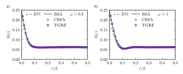
Figure 10: Comparison of the two-point correlations for the three types of microstructures (RSA, CRSA and TGRF), with c = 25% and various values of  $\omega$ . (a)  $\omega = 0.2$ . (b)  $\omega = 1$ . For the CRSA microstructures,  $\eta = 0.3$  and  $\zeta = 6$ .
