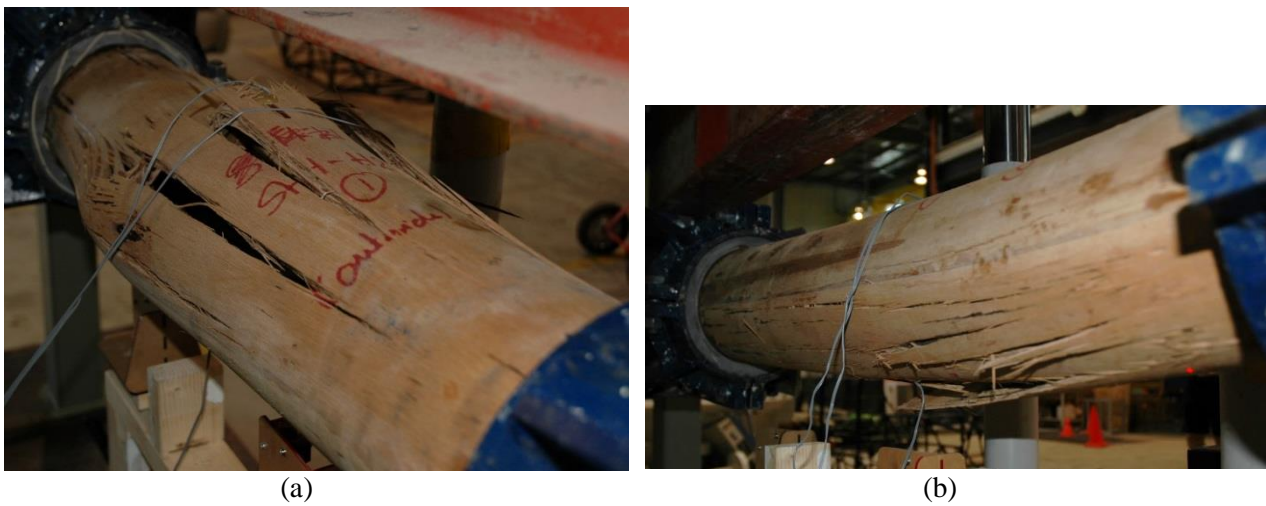
Figure 2: (a) Sudden compressive and (b) tensile failure modes in [1]
