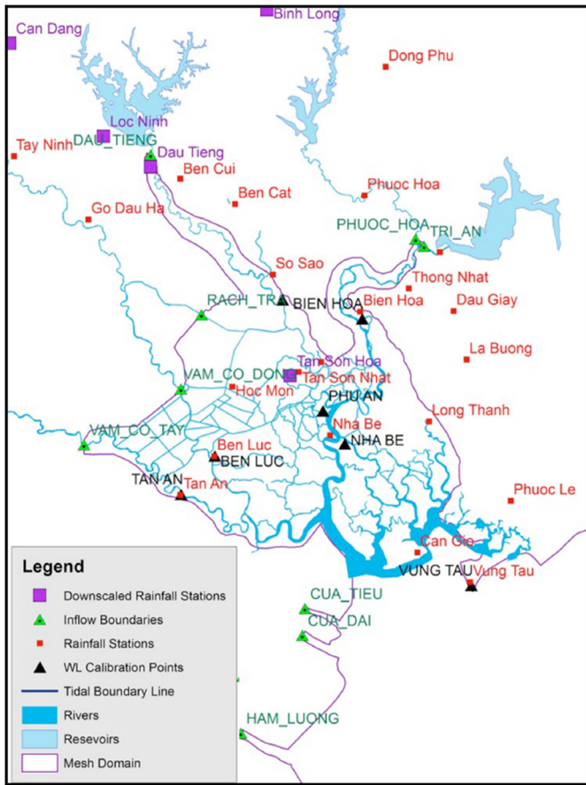
Fig. 7. Meteorological stations, calibration points and boundaries of Telemac2D model for lower SGDNB.
