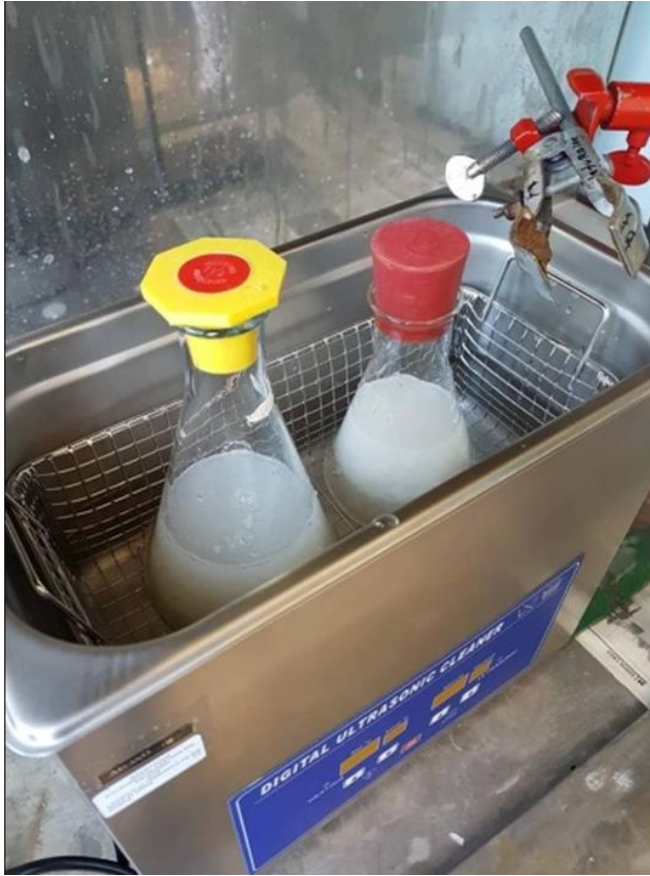
Figure 2. Ultrasonic bath for homogenization of BNC - distilled water mixture.
