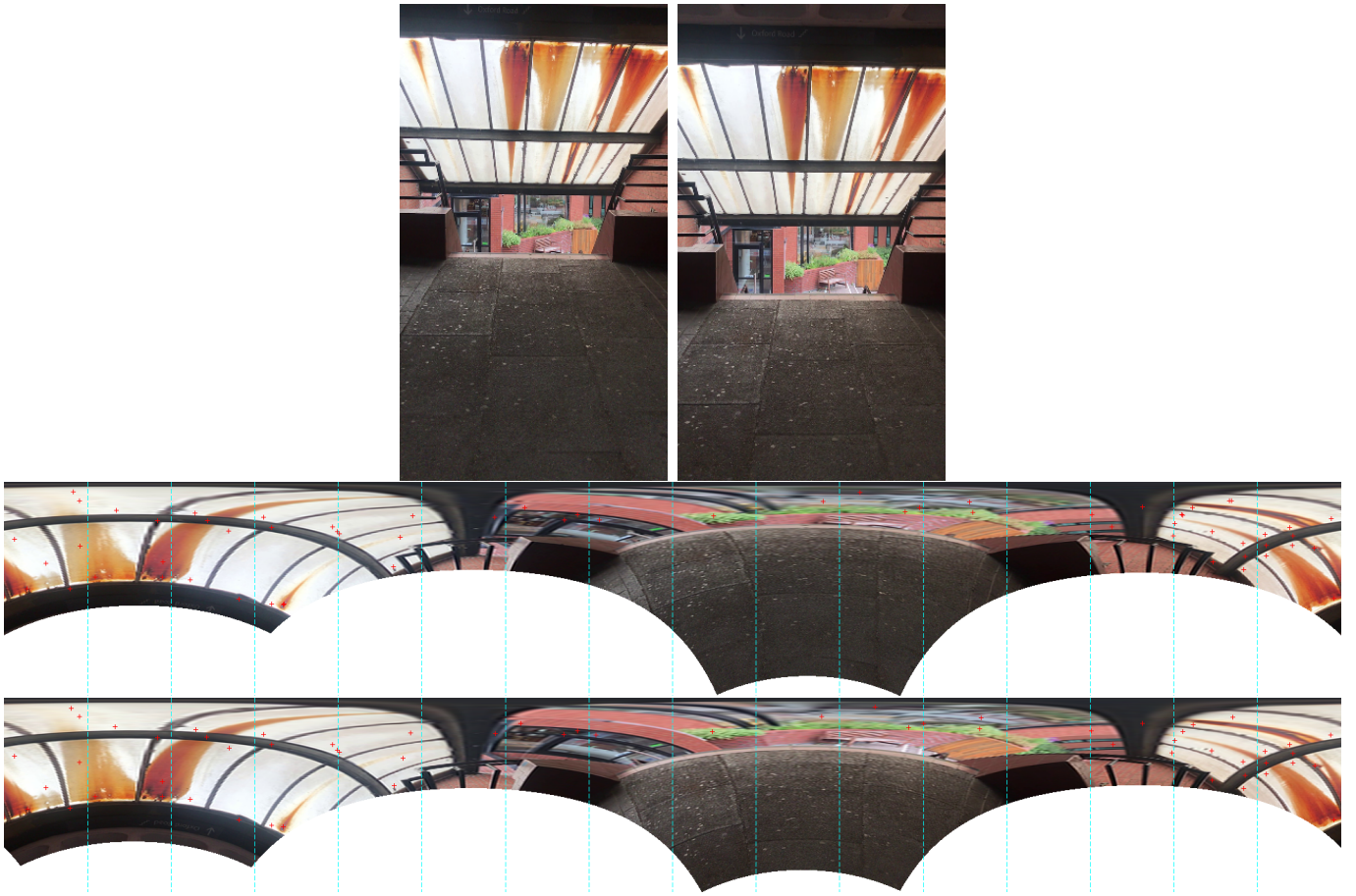
Figure 9: Polar rectification with epipoles inside the image. Rectified images are presented rotated for layout purposes, so that points move vertically.
