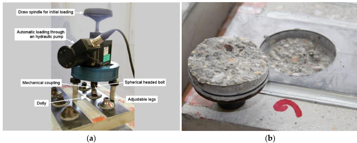
Figure 1. (a) Commercial pull-off tester; (b) typical cohesive failure in concrete substrate with pull-off strength of 5.9 MPa, demonstrating a sound bonded FRP system according to the standards.
