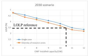
Fig. 2. Impact of offshore wind capacity to the Loss of Load Probability
