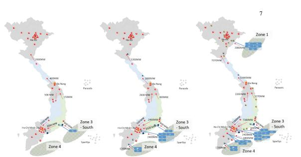
**Fig. 3.** Load flow snapshot in 2023, 2025 and 2030 (from left to right) - Cases of high renewable sources including max capacity from OWFs.
