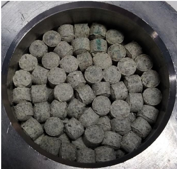
166 Figure 5: Pictures of SP0 samples. a) SP0a at 9 MPa of suction, b) SP0b following liquid water saturation. The cell 167 diameter is 60 mm.
