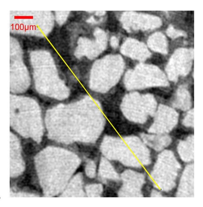
Figure 9. Example of image of MHBS obtained with the setup No. 1. Voxel size:  $5\mu m$ .
