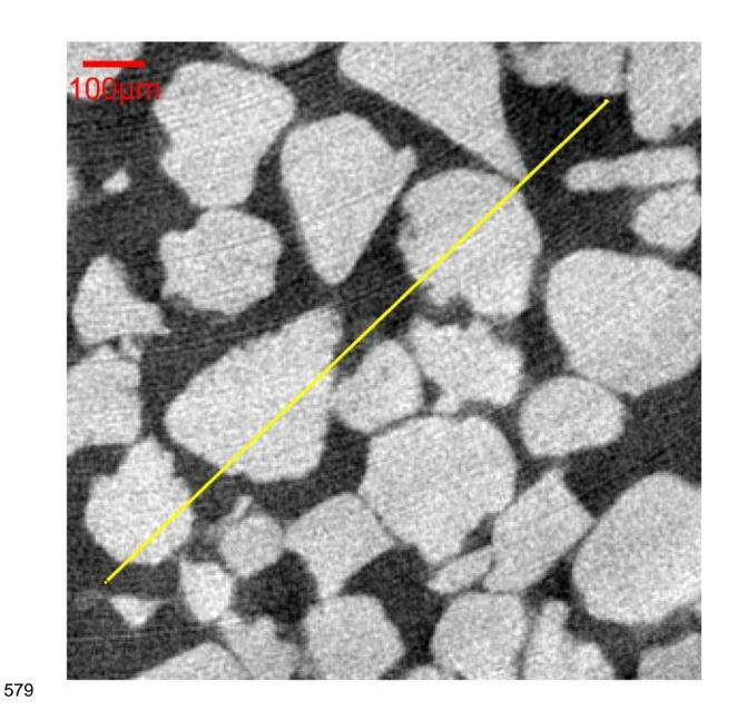
Figure 12. Example of image of MHBS obtained with the setup No. 2. Voxel size: 3,5  $\,\mu m.$
