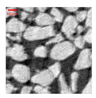
Figure 8. Example of image of an unsuccessful scan due to the cell vibration, obtained with the experimental setup No. 1. Voxel size: 5µm.
