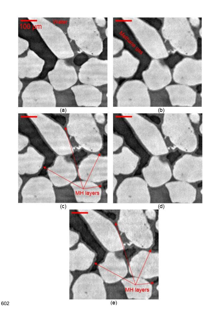
Figure 19. Vertical cross-section showing the MH formation (tap water) at: (a) t = 0.3
