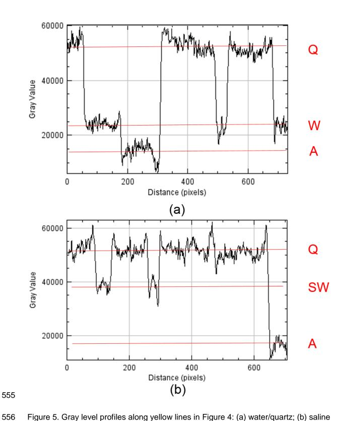
Figure 5. Gray level profiles along yellow lines in Figure 4: (a) water/quartz; (b) saline water/quartz.
