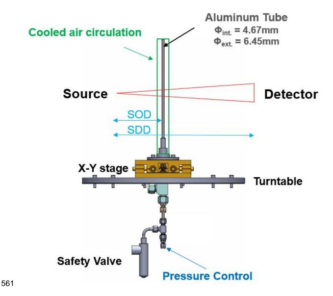
Figure 6. Experimental setup principles for XRCT scans of MHBS. SOD: Source Object Distance; SDD: Source Detector Distance.
