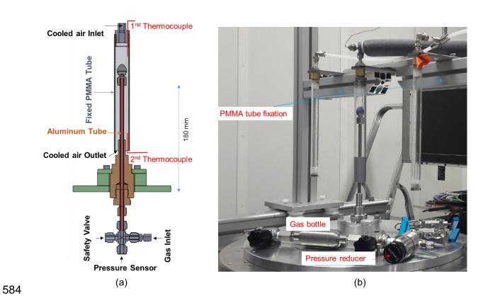
Figure 14. Experimental setup No. 3: (a) Schematic view; (b) picture.
