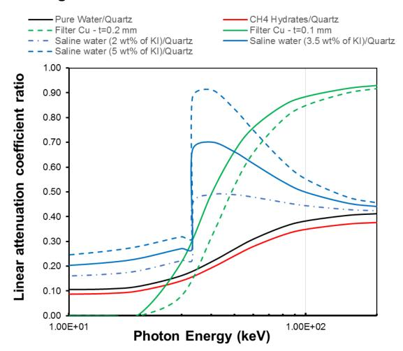
546 Figure 1. Linear attenuation coefficient ratio between phases, and X-Ray transmission through Cu filter, versus photon energy.
