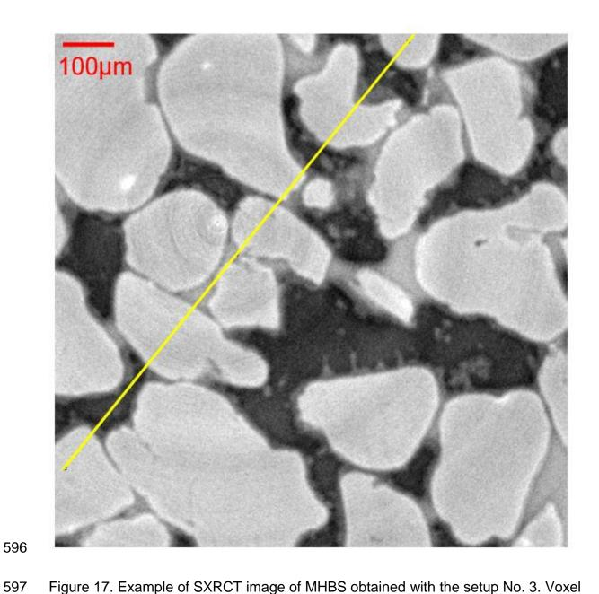
Figure 17. Example of SXRCT image of MHBS obtained with the setup No. 3. Voxel size: 0.9  $\mu m. \,$
