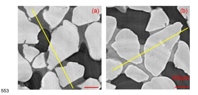
Figure 4. SXRCT images of unsaturated sand with (a) pure water; (b) saline water.
