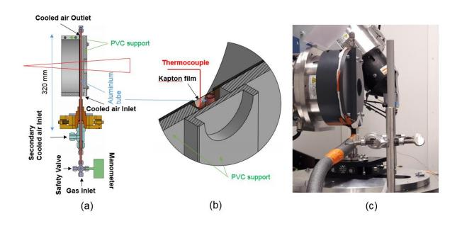
Figure 11. Experimental setup No. 2: (a), (b) Schematic view; (c) picture.
