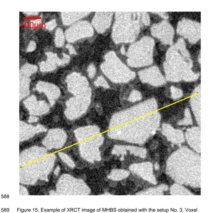
Figure 15. Example of XRCT image of MHBS obtained with the setup No. 3. Voxel size: 4  $\mu m. \,$
