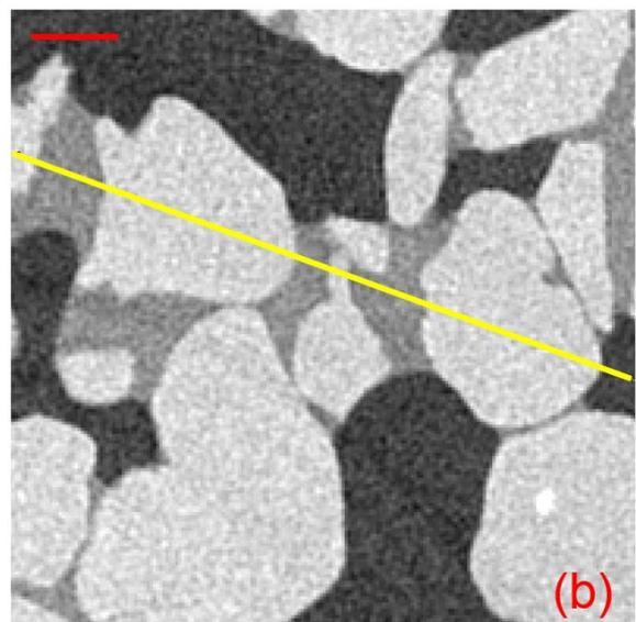
549 Figure 2. XRCT images of unsaturated sand with (a) pure water; (b) saline water.
