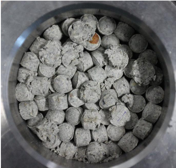
Fig. 10b Picture of the SP2 sample after dismantling at 9 MPa of suction. The cell diameter is 60 mm
