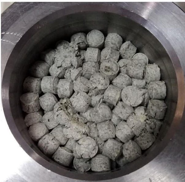
Fig. 10b Picture of the SP2 sample after dismantling at 9 MPa of suction. The cell diameter is 60 mm
