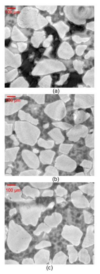
Figure 16. Possible morphologies and pore habits of MHs: (a) image in Z-3 (t = 19 h); (b) image in Z1 (t = 19.5 h; (c) image in Z-1 (t = 19.2 h).
