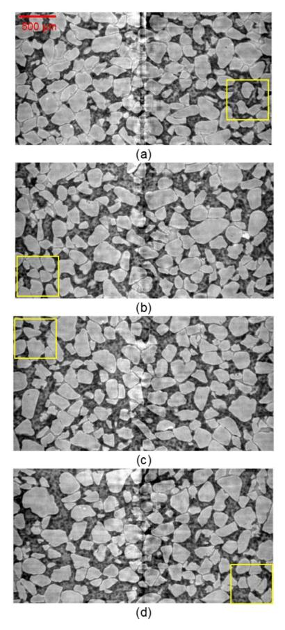
Figure 14. Vertical cross-section through Z9 (a, t = 20.5 h), Z7 (b, t = 20.2 h), Z5 (c, t = 20 h) and Z3 (d, t = 19.7 h). Image dimensions: 3.47 mm x 1.75 mm.
