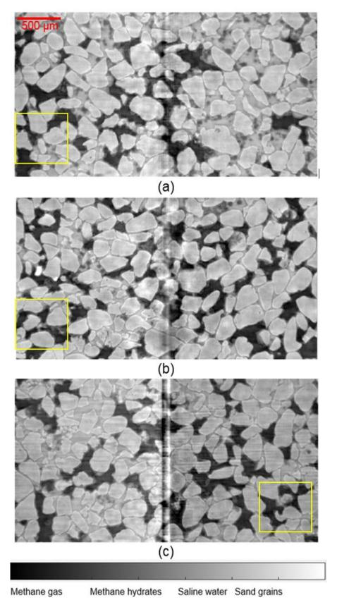
Figure 12. Vertical cross-section through Z-3 (a, t = 19.0 h), Z-5 (b, t = 18.8 h), and Z-7 (c, t = 18.5 h). Image dimensions: 3.47 mm x 1.75 mm.
