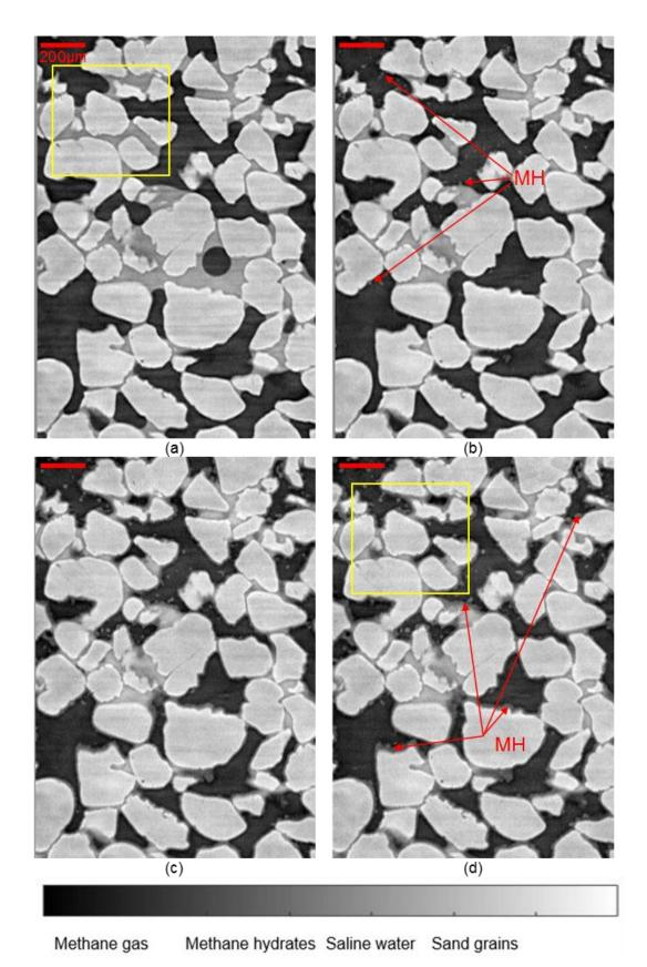
Figure 4. Vertical cross-section through Z0\_HR: (a) t = 0; (b) t = 0.58 h; (b) t = 4 h; (c) t = 4.5h.
