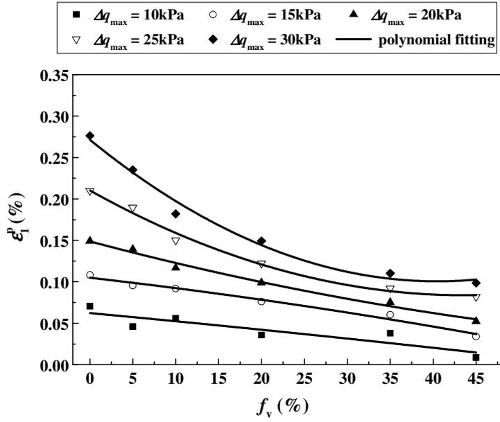
Fig. 3. Polynomial fitting of end-stage permanent strain  $\varepsilon_1^p$  with  $f_v$  at different  $\Delta q_{max}$  values
