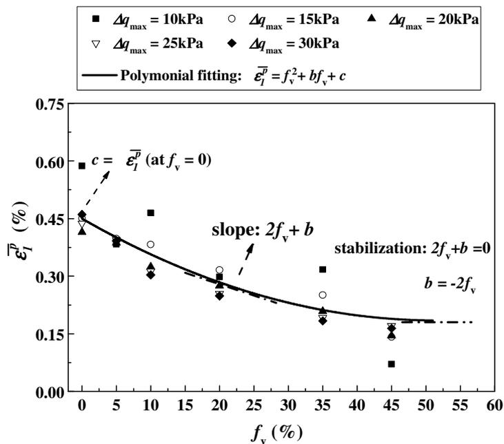
Fig. 10. Variations of end-stage permanent strain  $\bar{\epsilon}_1^p$  with coarse grain content  $f_v$
