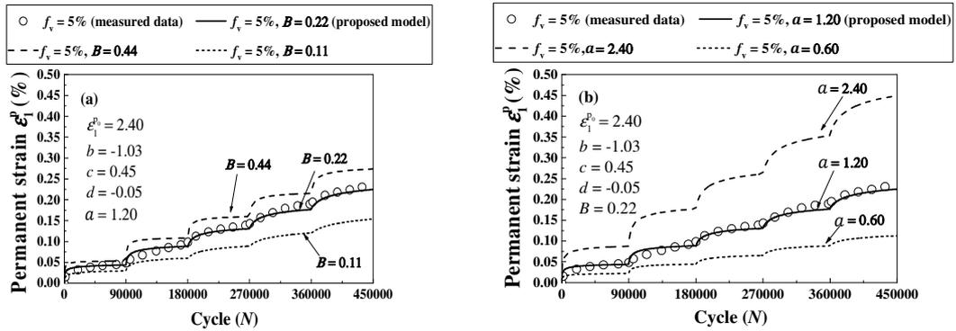
Fig. 9. Effects of parameters  $a$  and  $B$  in  $h(N)$  on the evolution of permanent strain with loading cycles  $N$ : (a) parameter  $B$ ; (b) parameter  $a$
