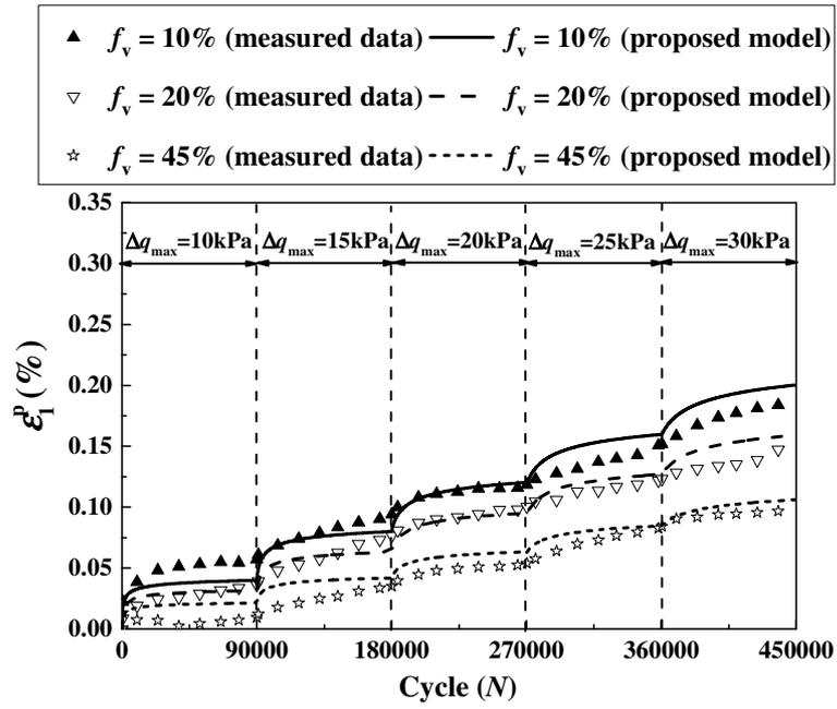
Fig. 11. Simulations of the cyclic test results by the proposed model for  $f_v = 10\%$ ,  $20\%$  and  $45\%$
