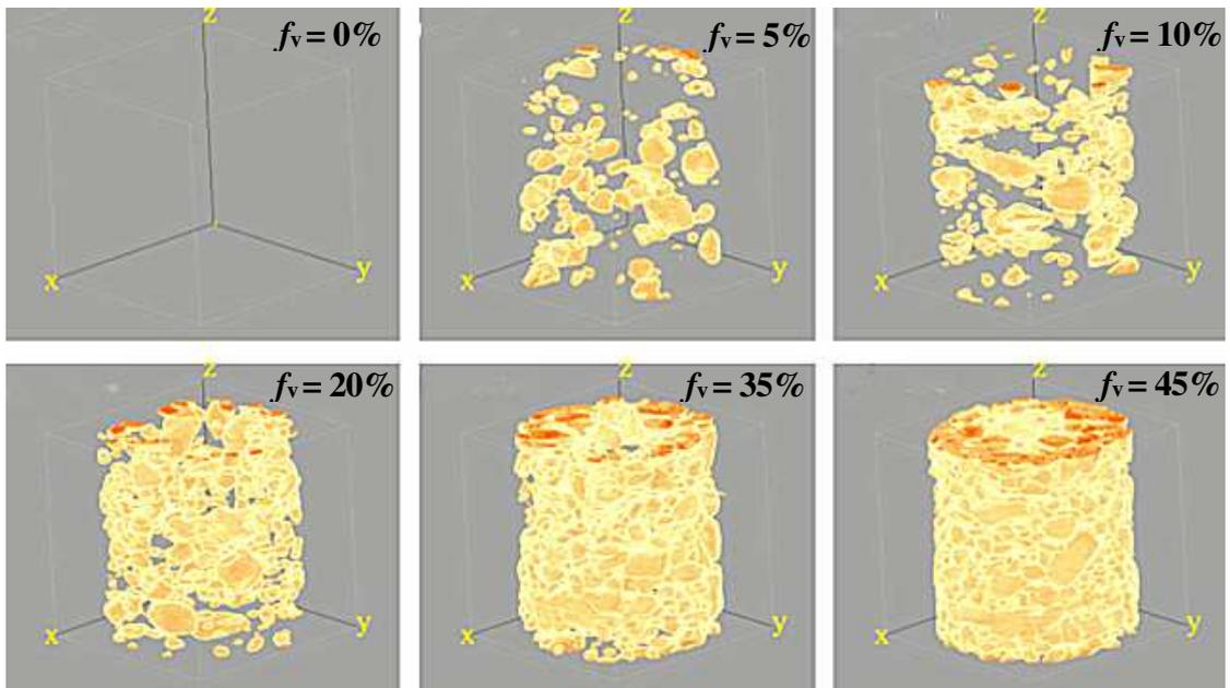
Fig. 2. 3D views of the coarse grain distributions in compacted samples (after Wang et al. 2018c)
