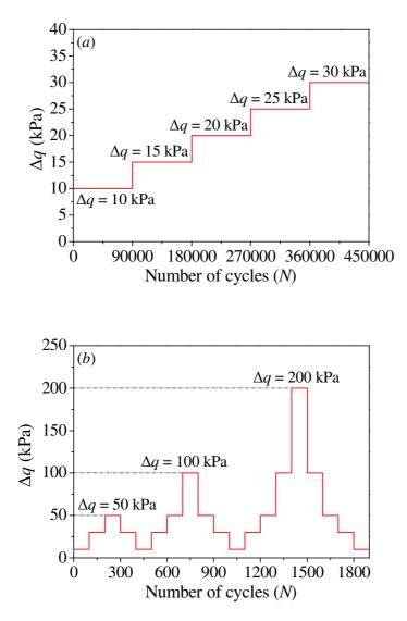
Fig. 4. Loading paths in two stages: (a) stage 1 for permanent strain investigation; (b)
