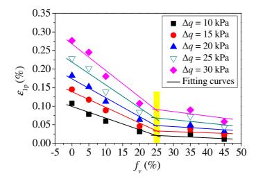
Fig. 10. Variations of estimated end-stage permanent strains with  $f_v$  at different stress
