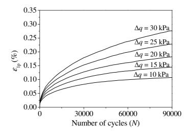
Fig. 9. Estimated permanent strain evolutions at the first 90,000 cycles for ballast
