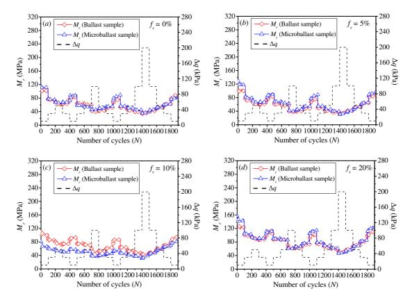
Fig. 18. Comparison of  $M_r$  value between ballast specimens and microballast
