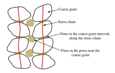
Fig. 17. Schematic illustration of the distribution of fines soils in case of grain-grain
