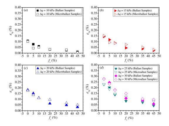
Fig. 16. Variations of estimated end-stage permanent strains with  $f_v$  for ballast and microballast specimens at: (a)  $\Delta q = 10$  kPa; (b)  $\Delta q = 15$  kPa; (c)  $\Delta q = 20$  kPa; (d)  $\Delta q$
