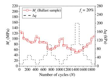
Fig. 14. Evolution of  $M_r$  with number of cycles at different stress levels for ballast
