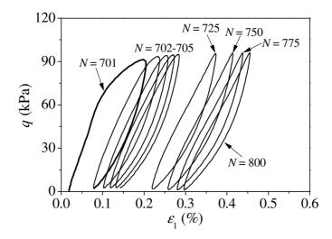
Fig. 12. Hysteresis loops during 100 cycles (N = 701 to 800) under  $\Delta q = 100$  kPa for
