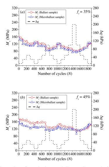
Fig. 19. Comparison of  $M_r$  value between ballast specimens and microballast specimens in case of grain-grain contact structure for (a)  $f_v = 35\%$  and (b)  $f_v = 45\%$
