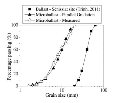
Fig. 1. Grain size distributions of the ballast and the microballast (modified from
