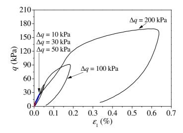
Fig. 11. Hysteresis loops at the first cycles of different stress levels for ballast
