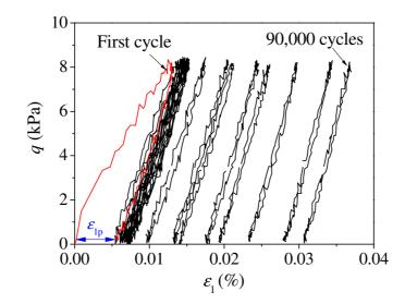
Fig. 5. Deviator stress q versus axial strain  $\varepsilon_1$  for the first 90,000 cycles of loading
