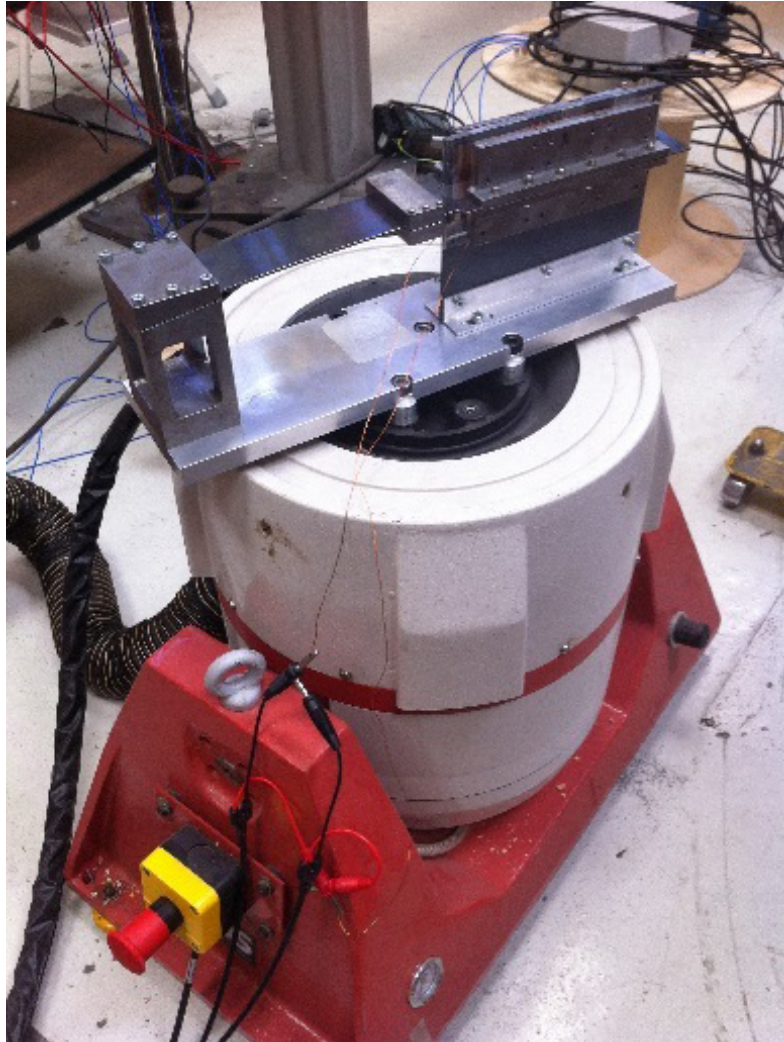
FIG. 20. Laboratory test of the harvester with an harmonic excitation.
