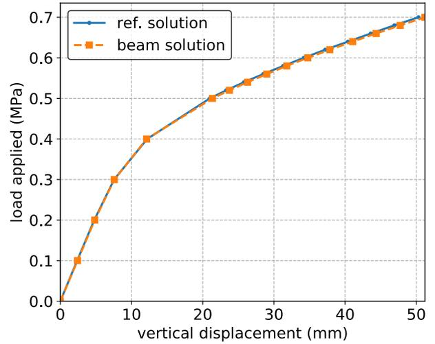
**Fig. 14** Maximum vertical displacement at mid-span of the beam
