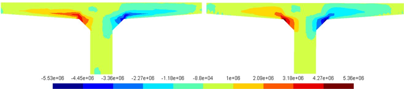
(d)  $\sigma_{12}$  computed from the beam solution (left) and from the reference solution (right)**Fig. 16** Stress computed at mid-span of the beam ( $x_3 = 5$  m) from the beam solution and the reference solution
