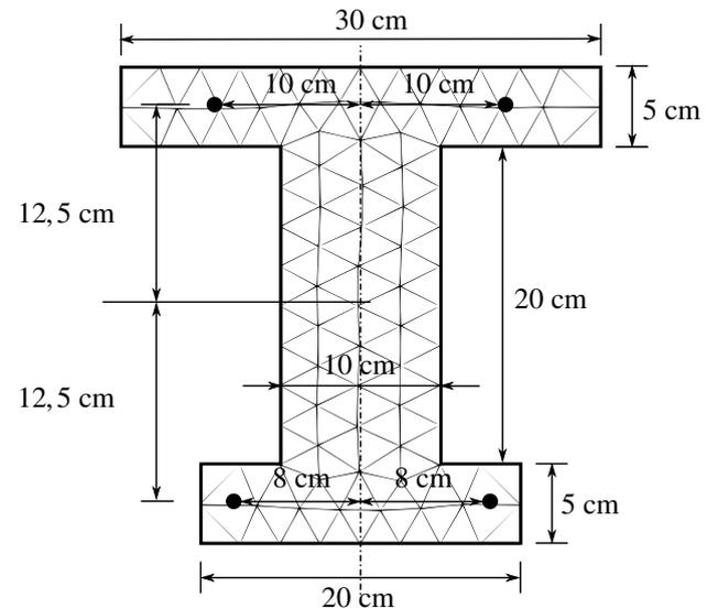
**Fig. 25** Geometry and mesh of the I-section
