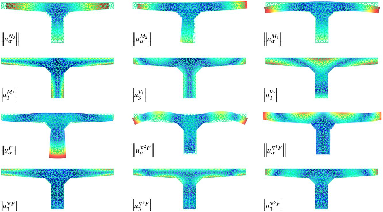
**Fig. 7** The 6 Saint Venant displacement modes ( $N_3$  longitudinal traction,  $M_\alpha$  Bending moments,  $M_3$  torsion warping,  $V_\alpha$  shear forces warping) and the 6 modes specific to the applied load.
