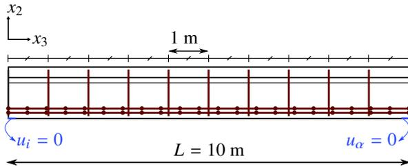
**Fig. 5** Boundary conditions and reinforcement of the T-beam
