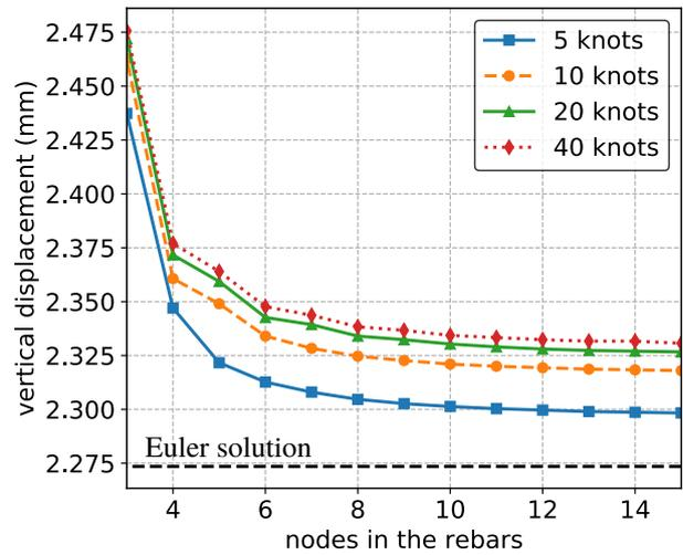
**Fig. 26** Maximum vertical displacement for different meshes refinements
