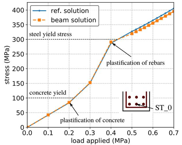
**Fig. 15** Stress in ST\_0 at mid-span as function of the load applied
