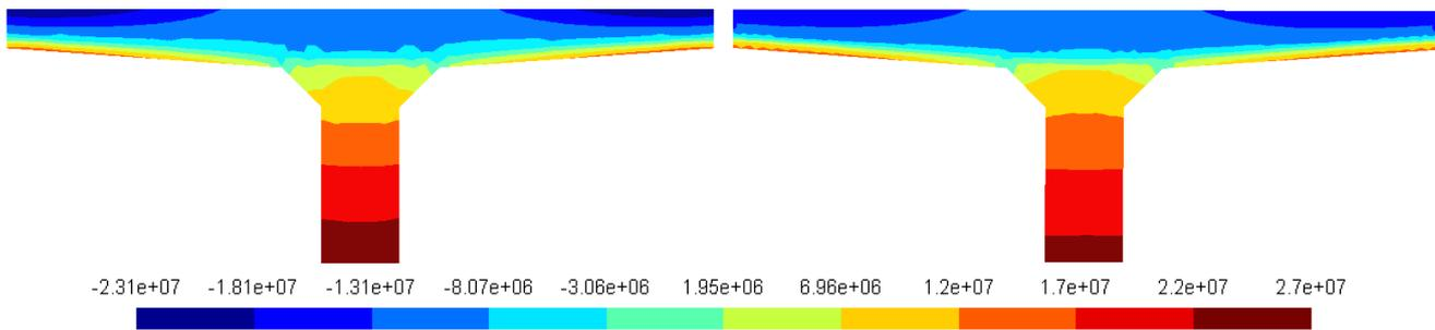
(c)  $\sigma_{33}$  computed from the beam solution (left) and from the reference solution (right)
