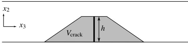
**Fig. 23** Definition of the potential cracked area
