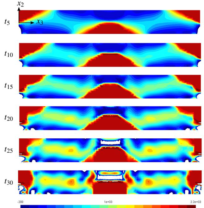
**Fig. 21** Evolution of maximum stress eigenvalues in the concrete body (in kPa)
