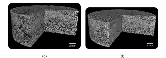
Figure 4: 3D reconstructed images of the sample at different compaction levels. (a) S1, (b) S2,
