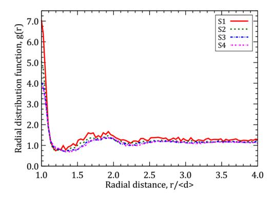
558 Figure 20: Radial distribution functions for particle centers of four compaction levels.
