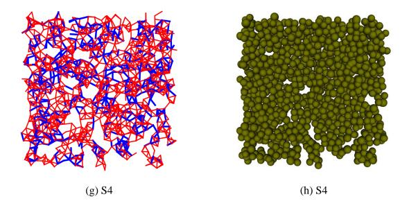
591 Figure 21: Contact network and reconstructed 3D image of a typical slice under growing of592 compaction level.
