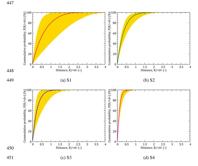
452 Figure 15: Pore distance distribution for four compaction levels. In each level, gold region453 denotes the values of ten cubes; continuous line denotes the average value.
