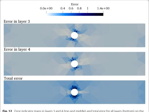
Fig. 12 Error indicator maps in layers 3 and 4 (top and middle) and total error for all layers (bottom) on the initial mesh
