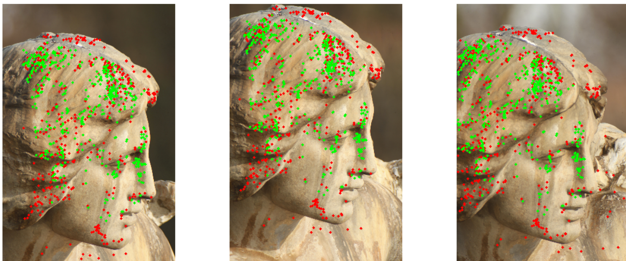
Figure 11: A triplet of images from a statue in Château de Champs. The matches are drawn in green if they are considered inliers by the orthographic AC-RANSAC and red otherwise.
