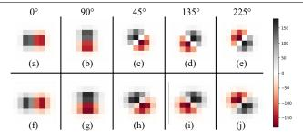
Figure 2: Steerable filters. Fig.(a-e) initial value ( $\alpha, \beta, l = 1$ ) Fig. (f-j) filters after training ( $\alpha = 0.43, \beta = 0.85, l = 1.12$ ). 45°, 135°, 225° are created by the linear combination of the basis filters on 0° and 90° using Eq. 5.
