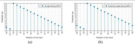
Figure 6: Co-variant relation between input rotation and output rows. The input (number 2) is rotated in  $d\phi$  steps. (a) Up-right training. (b) Randomly rotated training.
