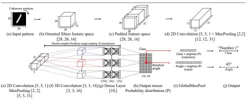
Figure 5: CNN Architecture using  $\Phi = 16$  and input image size of [28, 28]. Output size of each layer between brackets. Upper-side is the feature extraction. Lower-side shows the shared predictor stage.
