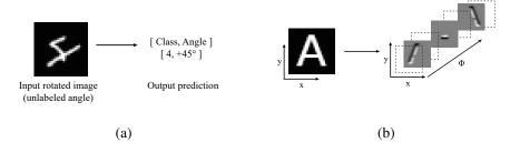
Figure 1: (a) Prediction of class and rotation angle. (b) Projection into roto-translational space.
